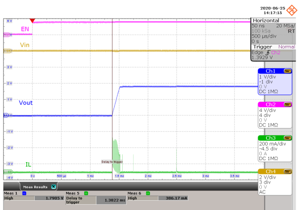
Figure 8-27. Load Transient, 300 mA Step
