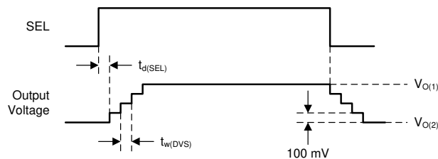
Figure 7-10. Dynamic Voltage Scaling with High Load
