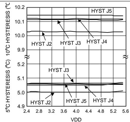
Figure 8. Line Regulation: Hysteresis vs Supply Voltage 30°C
