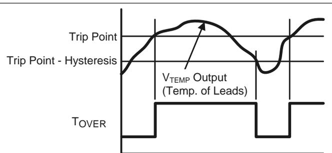
Figure 23. Output Transfer Characteristic
