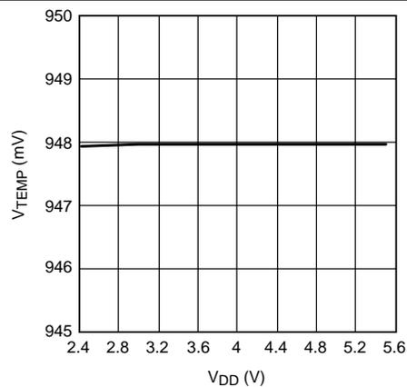
Figure 7. Line Regulation:  $V_{TEMP}$  vs Supply Voltage
