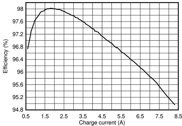
**Figure 7-3. Battery Charge Efficiency vs. Charge Current, 2 x 22- $\mu$ F CFLY per Phase**
