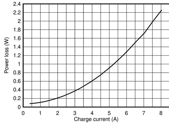
**Figure 7-2. Battery Charge Power Loss vs. Charge Current, 1 x 22- $\mu$ F CFLY per Phase Switching Frequency**
