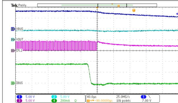
Figure 9-5. Adapter Unplug in Switched Cap Mode
