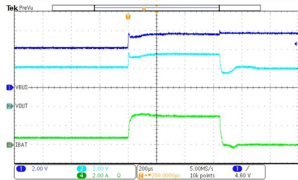
**Figure 9-14. IBATOCP in Bypass Mode**
