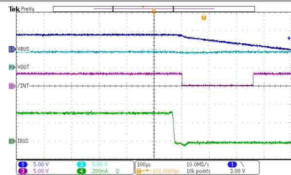
Figure 9-6. Adapter Unplug in Bypass Mode
