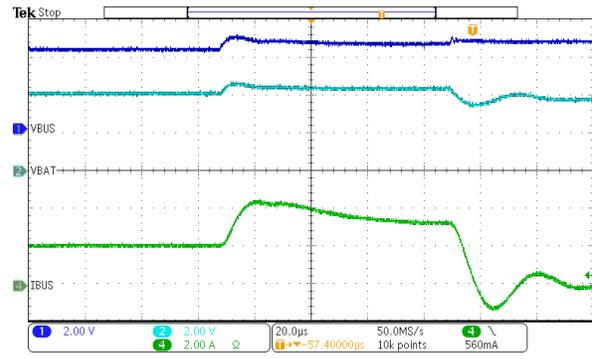
**Figure 9-10. IBUSOCP in Bypass Mode**
