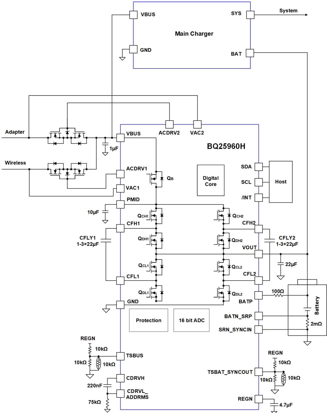
Figure 9-1. BQ25960H Typical Application Diagram with Dual Input
