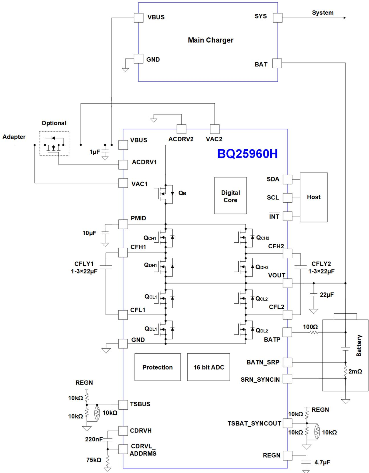
Figure 9-2. BQ25960H Typical Application Diagram with Single Input
