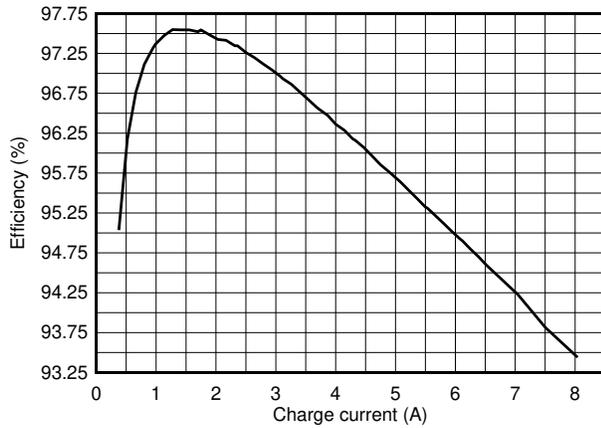
**Figure 7-1. Battery Charge Efficiency vs. Charge Current, 1 x 22- $\mu$ F CFLY per Phase Switching Frequency**
