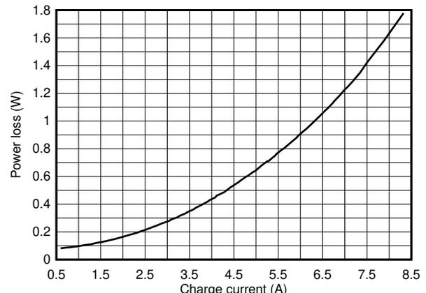
**Figure 7-4. Battery Charge Power Loss vs. Charge Current, 2 x 22- $\mu$ F CFLY per Phase**
