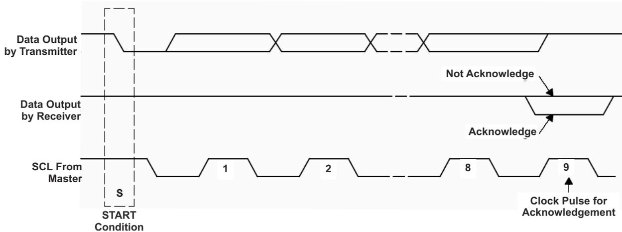
**Figure 8-12. Acknowledge on the I<sup>2</sup>C BUS**
