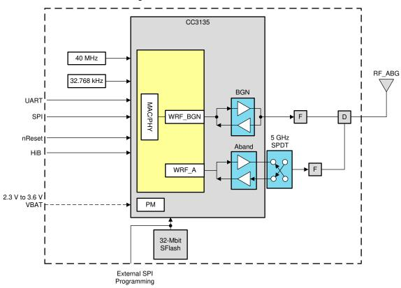
Figure 4-1. CC3135MOD Module Functional Block Diagram
