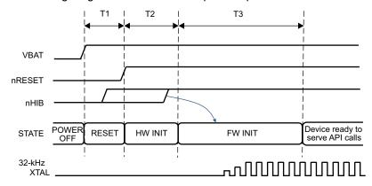
Figure 8-6. First-Time Power-Up and Reset Removal Timing Diagram
