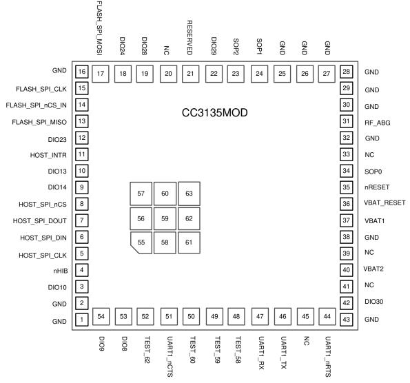
Figure 7-1 shows the approximate location of pins on the module.
