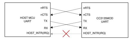
Figure 8-11. 4-Wire UART Configuration
