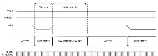
Figure 8-7. nHIB Timing Diagram
