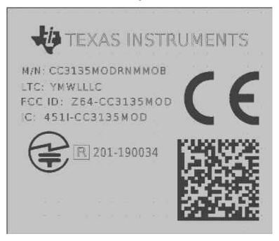
Figure 9-1. SimpleLink™ CC3135 Module Markings
