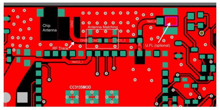
Figure 10-4. RF Section Layout
