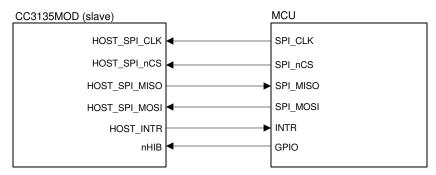
Figure 8-8. SPI Host Interface
