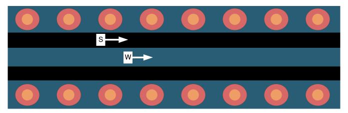
Figure 10-7. CPW With GND and Via Stitching (Top View)
