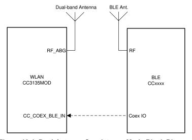
Figure 10-1. Dual-Antenna Coexistence Mode Block Diagram
