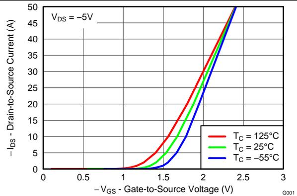
Figure 3. Transfer Characteristics
