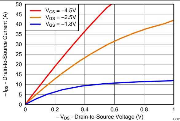
Figure 2. Saturation Characteristics
