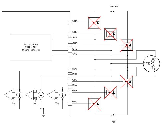
Figure 31. Offline Short-to-Supply Detection Circuit
