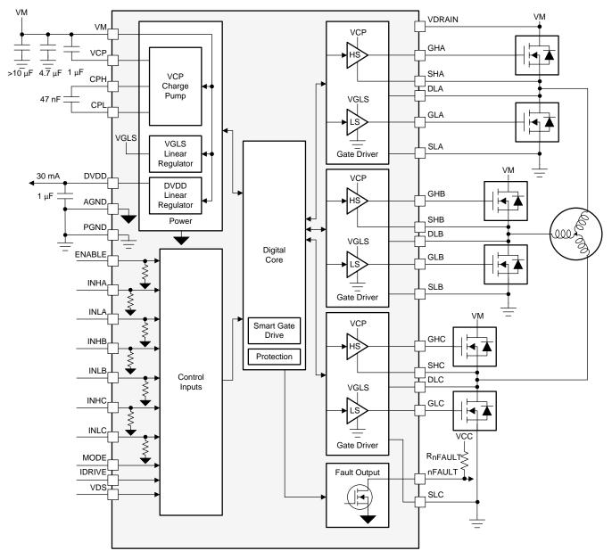
Figure 6. Block Diagram for DRV8340H
