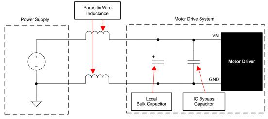
Figure 57. Motor Drive Supply Parasitics Example
