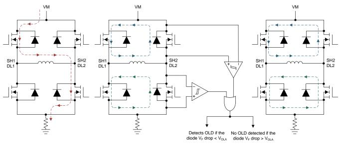
Figure 30. Circuit for Open Load Detection in Active Mode
