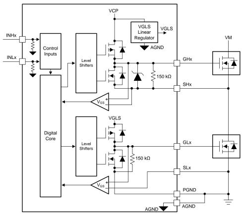
Figure 20. Gate Driver Block Diagram
