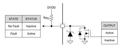
Figure 27. Open-Drain Output Pin Structure
