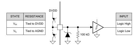
Figure 25. Logic-Level Input Pin Structure
