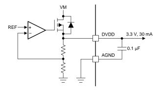
Figure 24. DVDD Linear Regulator Block Diagram
