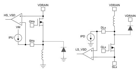
Figure 29. Load Configurations Not Supported
