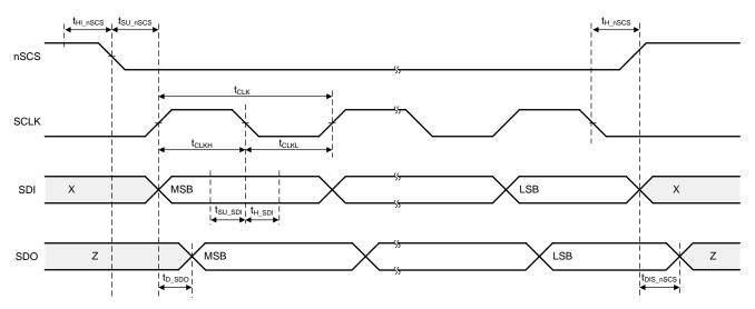
Figure 1. SPI Slave Mode Timing Diagram
