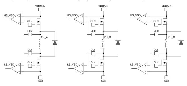
Figure 15. Solenoid Drive Configuration
