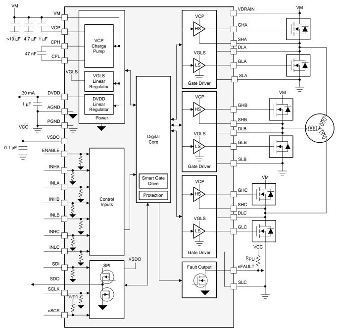
Figure 7. Block Diagram for DRV8340S
