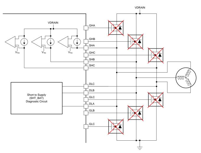
Figure 32. Offline Short-to-Ground Detection Circuit
