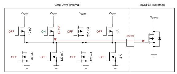
Figure 19. Charge Pump Architecture
