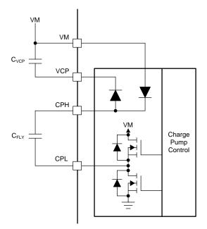
Figure 18. Charge Pump Architecture
