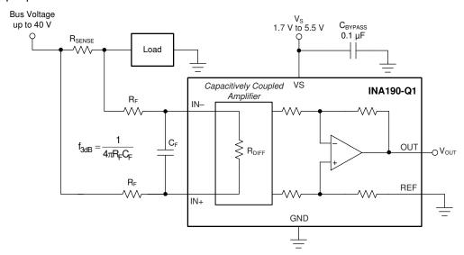
Figure 8-2. Filter at the Input Pins
