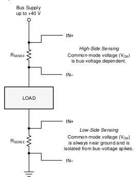
Figure 7-1. High-Side and Low-Side Sensing Connections
