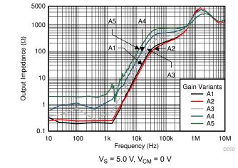
Figure 6-33. Output Impedance vs. Frequency
