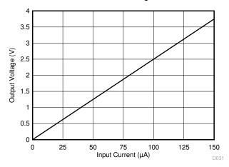
Figure 8-7. Typical Application DC Transfer Function
