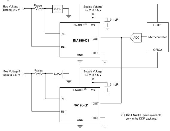
Figure 7-5. Multiplexing Multiple Devices With the ENABLE Pin
