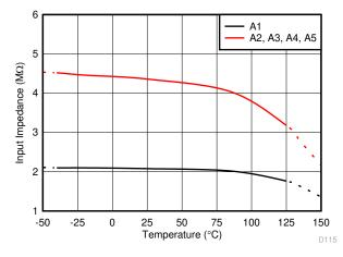
Figure 8-3. Differential Input Impedance vs. Temperature
