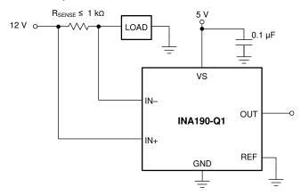
Figure 8-6. Microamp Current Measurement
