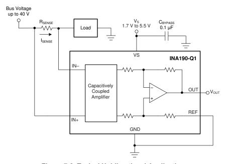
Figure 7-2. Typical Unidirectional Application
