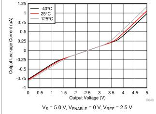
Figure 6-31. Output Leakage vs. Output Voltage (A1, A2, and A3 Devices)
