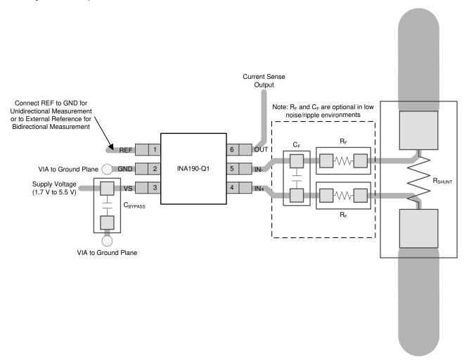
Figure 10-1. Recommended Layout for SC70 (DCK) Package
