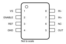
Figure 5-2. DDF Package 8-Pin Thin SOT-23 Top View
