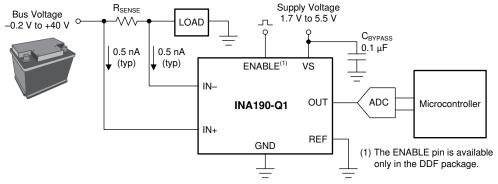
NOTE: To help eliminate ground offset errors between the device and the analog-to-digital converter (ADC), connect the REF pin to the ADC reference input. When driving SAR ADCs, filter or buffer the output of the INA190-Q1 before connecting directly to the ADC.
