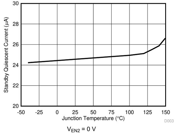
**Figure 7-8. Channel 1 Standby Current versus Temperature**
