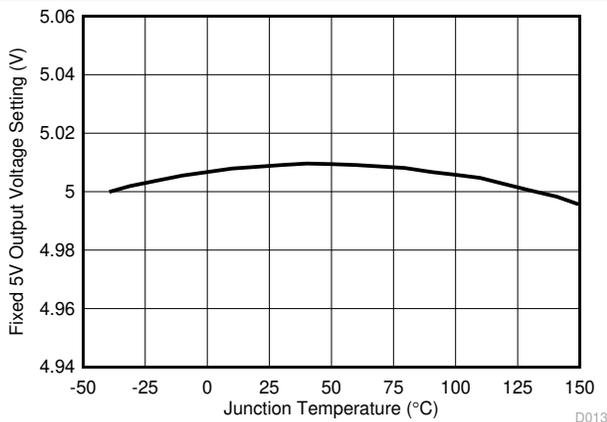
**Figure 7-11. Fixed 5-V Output Voltage (VOUT1) versus Temperature**
