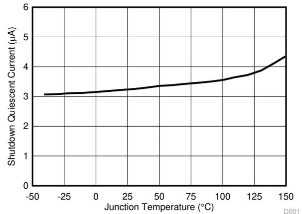
Figure 7-6. Shutdown Current versus Temperature
