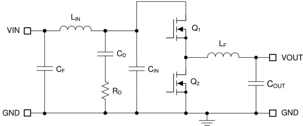
**Figure 9-2. Buck Regulator With  $\pi$ -Stage EMI Filter**
