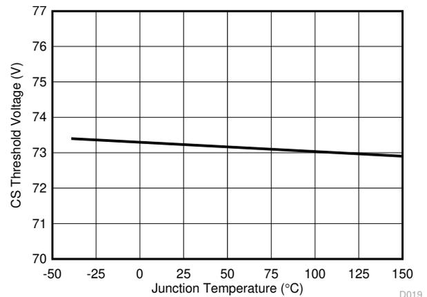
**Figure 7-22. Current Sense (CS1) Threshold versus Temperature**
