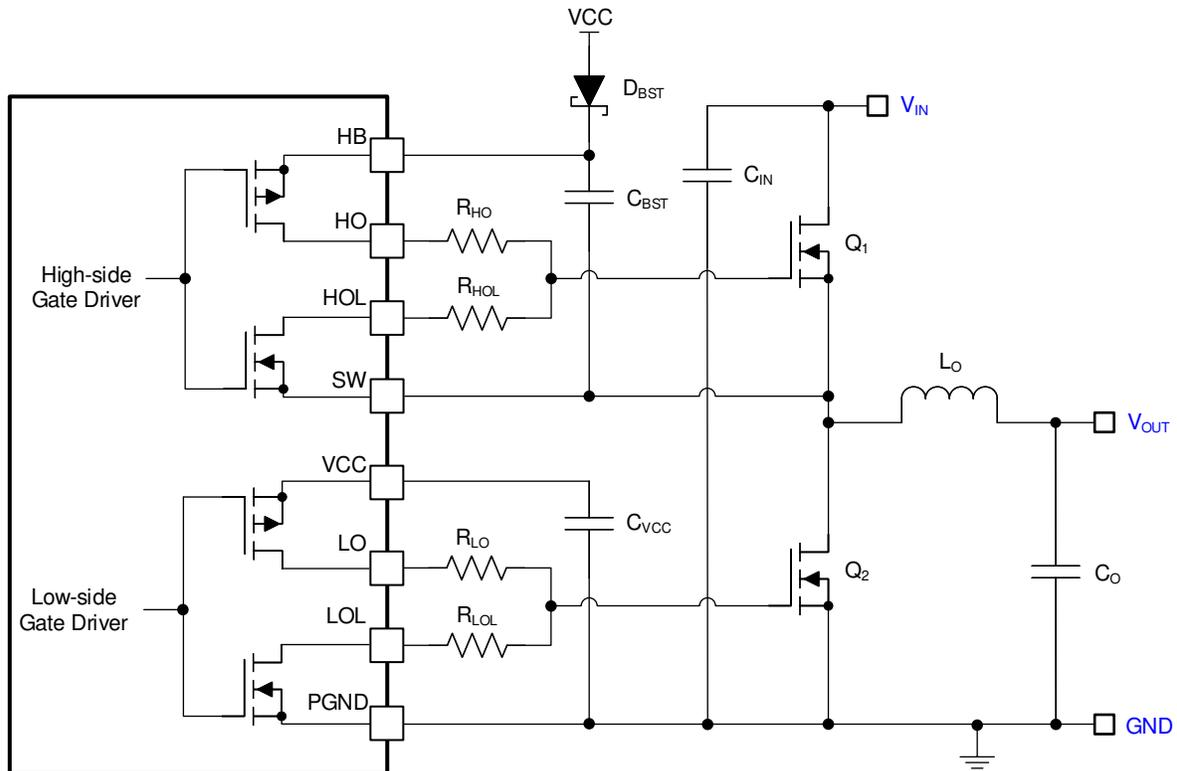
Figure 8-7. Integrated MOSFET Gate Drivers
