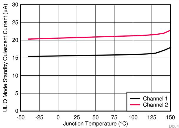
**Figure 7-9. ULIQ Mode Standby Current versus Temperature**
