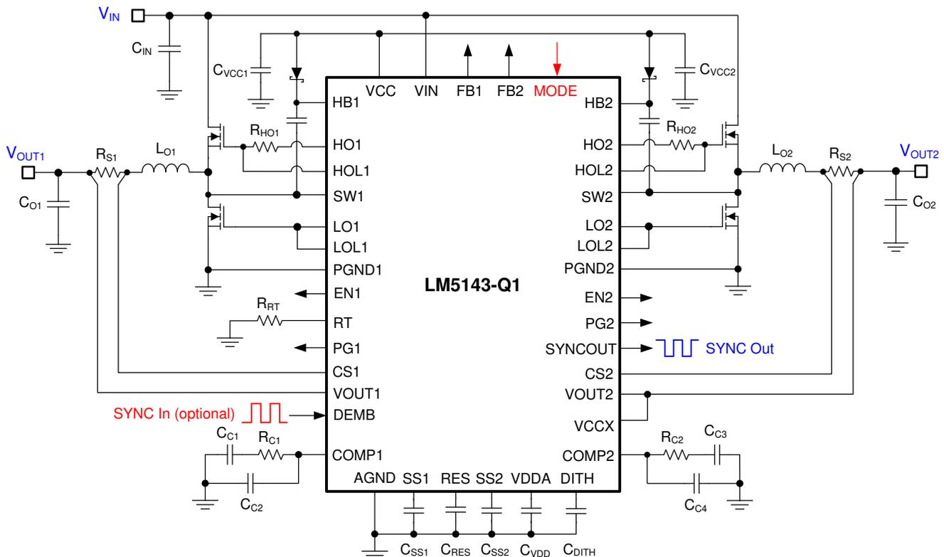
Figure 8-8. Regulator Schematic Configured for Independent Dual Outputs
