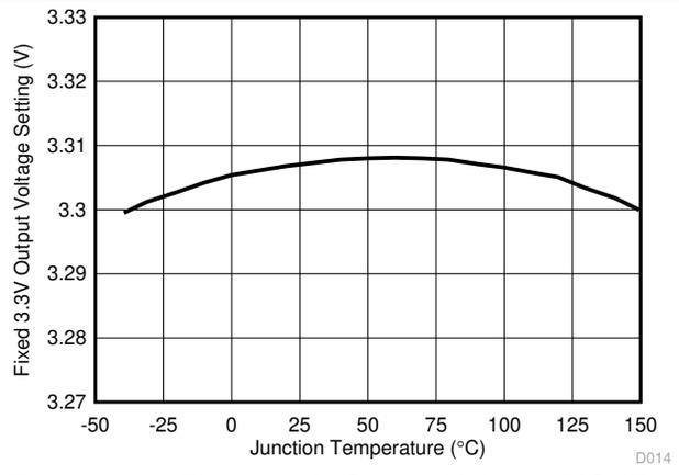
**Figure 7-10. Fixed 3.3-V Output Voltage (VOUT1) versus Temperature**
