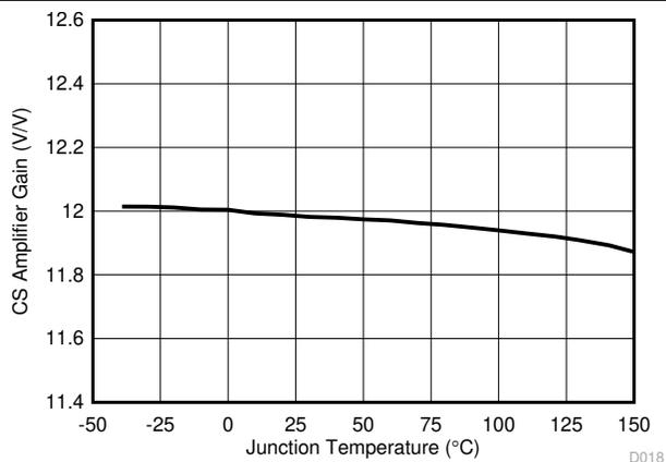
**Figure 7-23. Current Sense (CS1) Amplifier Gain versus Temperature**
