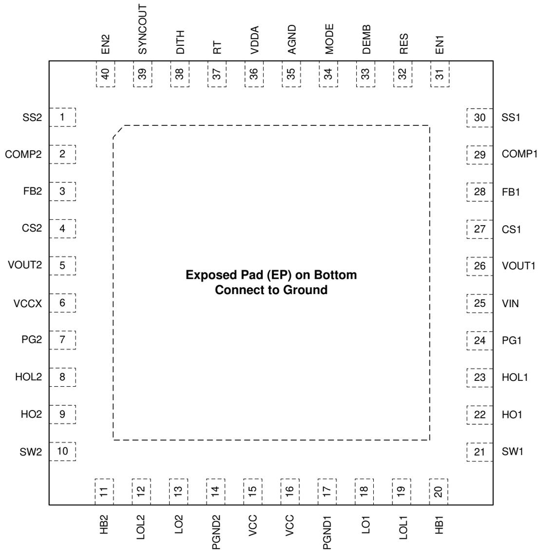
Connect Exposed Pad on the bottom to AGND and PGND on the PCB.
