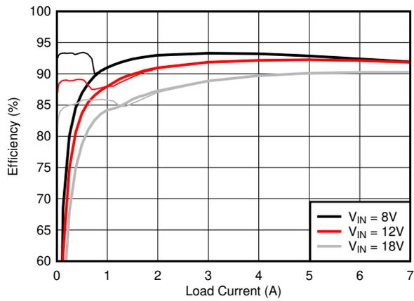
See Figure 9-4  $V_{OUT} = 5\text{ V}$   $F_{SW} = 2.1\text{ MHz}$
