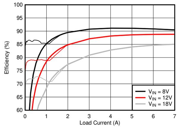
See Figure 9-4  $V_{OUT} = 3.3\text{ V}$   $F_{SW} = 2.1\text{ MHz}$
