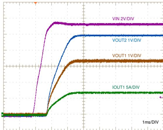
$V_{IN}$  step to 12 V      7-A resistive loads
