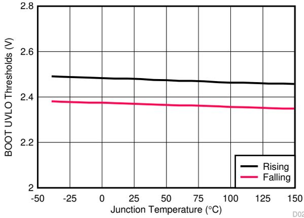
**Figure 7-25. BOOT (HB1) UVLO Thresholds versus Temperature**
