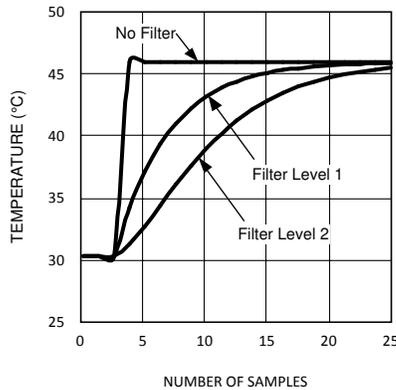
**Figure 6-5. Step Response of the Digital Filter**
