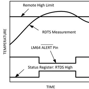
**Figure 6-2.  $\overline{\text{ALERT}}$  Output as Temperature Comparator Response Diagram**
