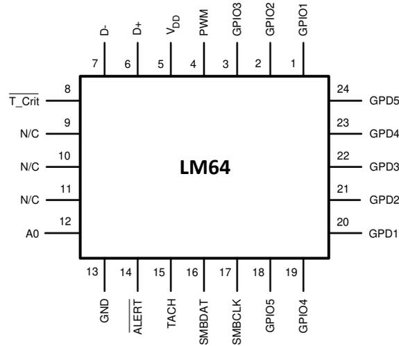
**Figure 4-1. 24-pin WQFN Package**
