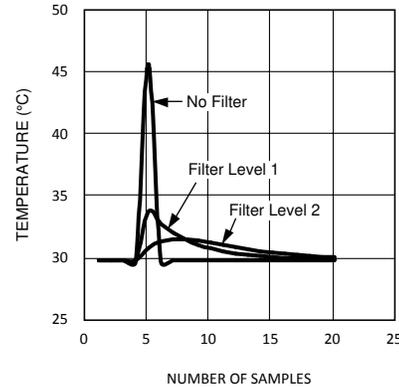
**Figure 6-6. Impulse Response of the Digital Filter**
