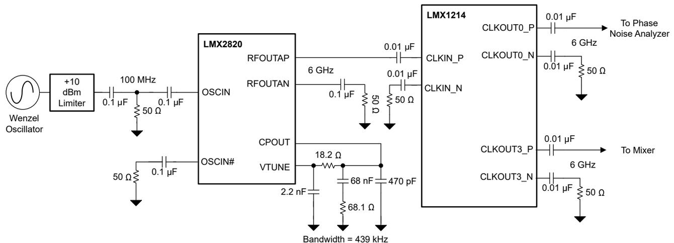
**Figure 7-6. Typical Application Schematic**
