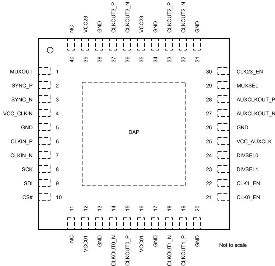
Figure 4-1. RHA0040C Package 40-Pin VQFN Top View
