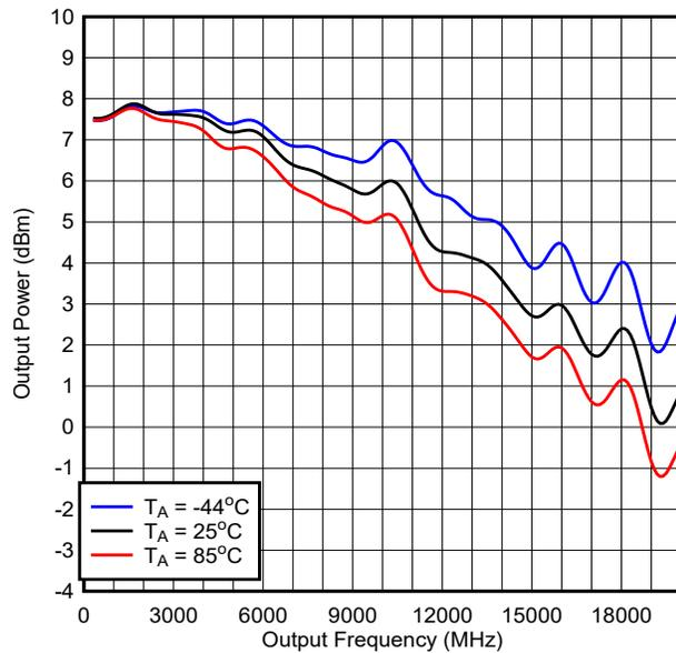
Figure 5-8. Buffer Mode Single-Ended Output Power Over Temperature
