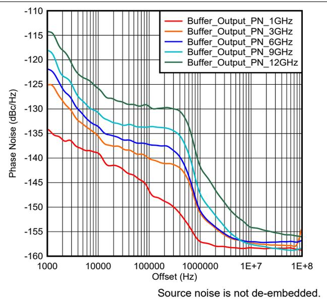
**Figure 5-3. Buffer Output Phase Noise Plots vs Output Frequencies**
