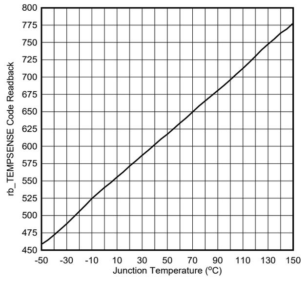
Figure 5-13. Temperature Sensor Readback
