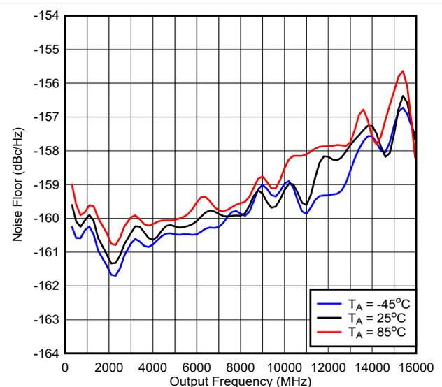
**Figure 5-5. Noise Floor in Buffer Mode**
