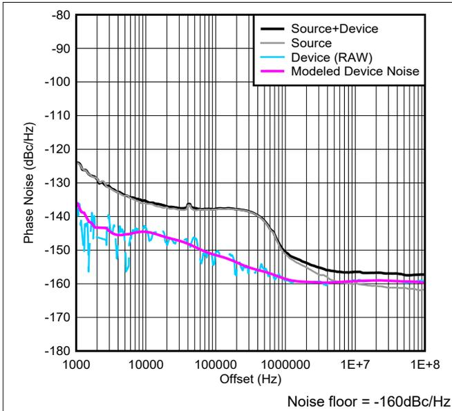
**Figure 5-2. Buffer Phase Noise Plot at 6-GHz Output**
