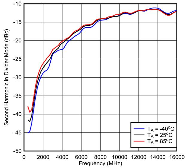
Figure 5-11. Second Harmonic in Divider Mode
