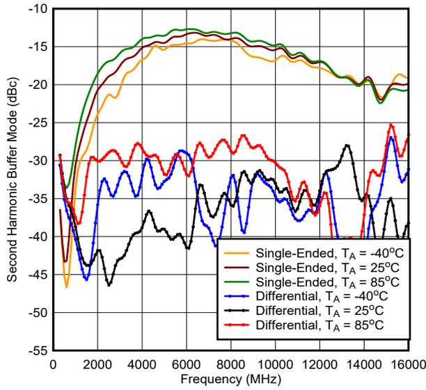
Figure 5-10. Second Harmonic in Buffer Mode
