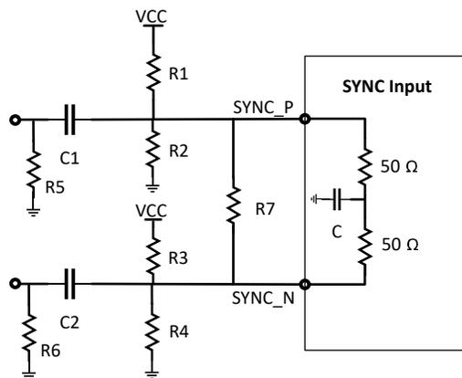
Figure 7-1. SYNC Input Circuit Recommendations
