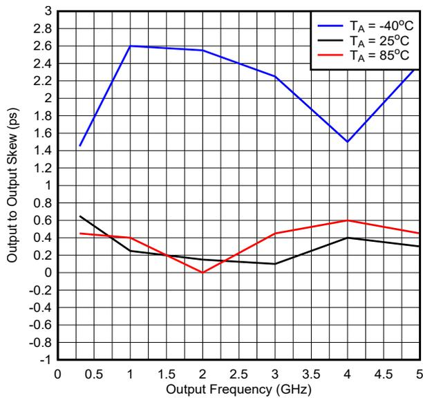
Figure 5-12. Output to Output Skew
