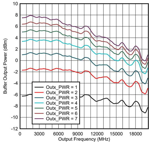
Applies to all modes except divider mode with odd divide (which will have slightly lower power).
