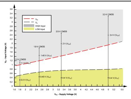
Figure 7-1. SCxT Input Voltage Levels
