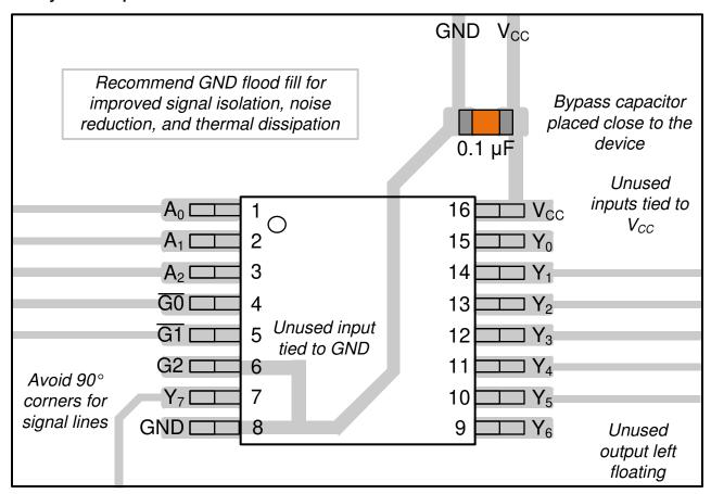
Figure 8-3. Example Layout for the SN54SC8T138-SEP
