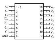
Figure 4-1. PW Package, 16-Pin TSSOP (Top View)
