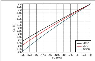
Figure 5-7. Output Voltage vs Current in HIGH State; 3.3-V Supply
