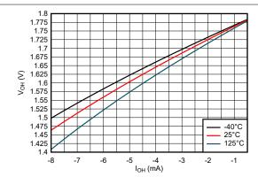
Figure 5-11. Output Voltage vs Current in HIGH State; 1.8-V Supply
