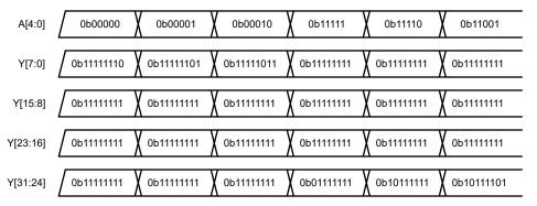
Figure 8-2. Application Timing Diagram
