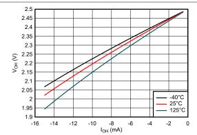
Figure 5-9. Output Voltage vs Current in HIGH State; 2.5-V
