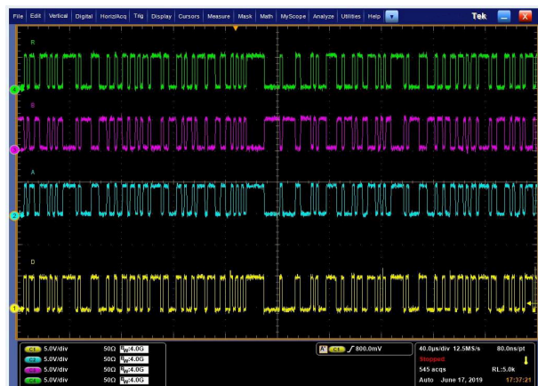
THVD2410 V_{CC} = 5\text{ V} R_L = 50\ \Omega Random (PRBS7) data at 500 kbps
