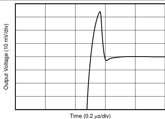
Figure 7-31. Small-Signal Step Response
