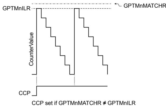
Figure 11-7 on page 693 shows how the CCP output operates when the  $PLO$  and  $MRSU$  bits are set and the **GPTMTnMATCHR** value is the same as the **GPTMTnILR** value. In this situation, if the  $PLO$  bit is 0, the CCP signal goes high when the **GPTMTnILR** value is loaded and the match would be essentially ignored.
