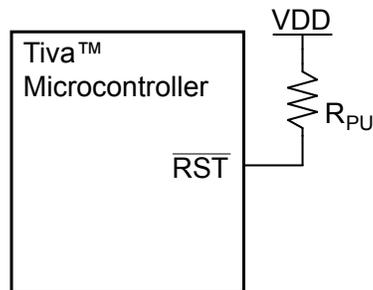
$R_{\text{PU}} = 0$  to 100 k $\Omega$
