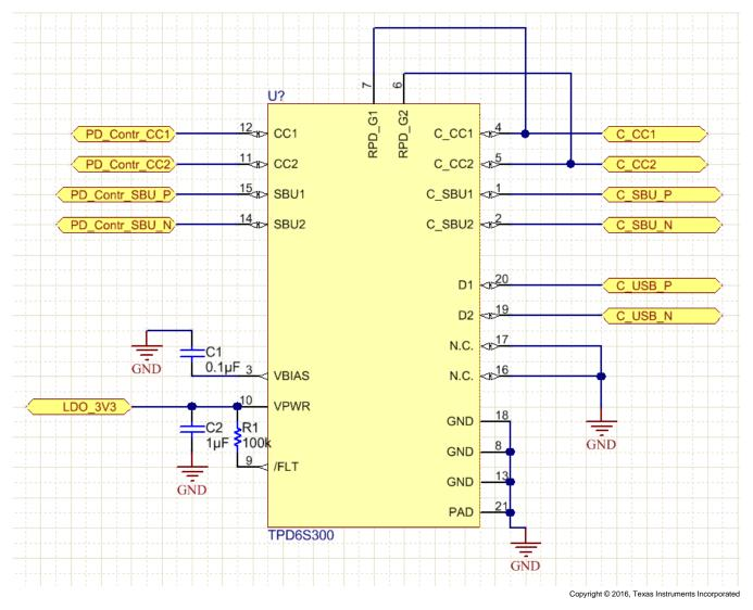
Figure 31. TPD6S300 Reference Schematic
