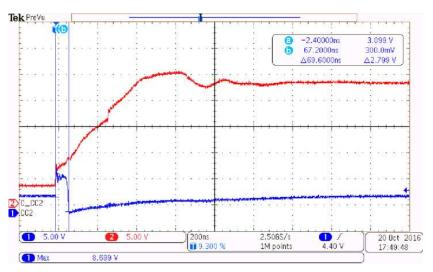
Figure 29. TPD6S300 Protecting the TPS65982 During a Short-to-V<sub>BUS</sub> Event
