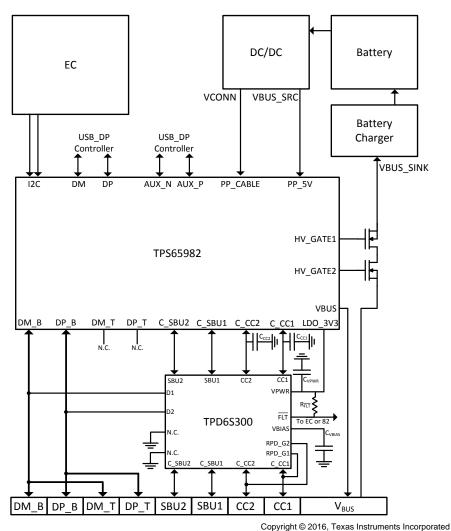
Figure 30. TPD6S300 Typical Application Diagram
