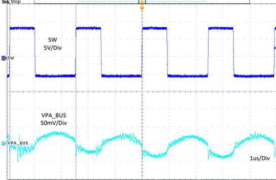
VSET = GND  $I_{PA\_BUS} = 0\text{ A}$   $I_{PB\_BUS} = 0\text{ A}$   $f_{SW} = 400\text{ kHz}$
