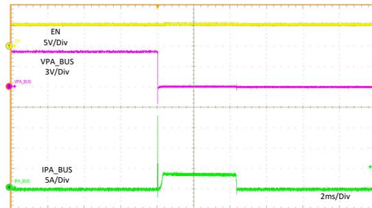
**Figure 11-26. VBUS Hot Short to GND**
