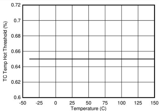
**Figure 8-24. TS Temperature Hot Threshold vs Junction Temperature**
