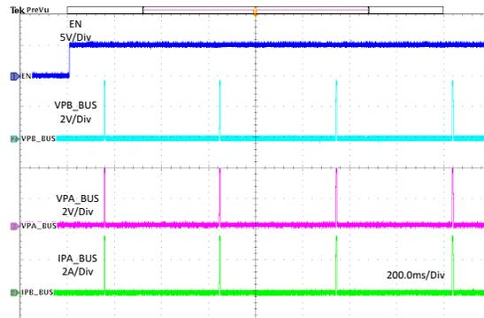
EN to High    PA\_BUS = 1  $\Omega$     PB\_BUS = 1  $\Omega$
