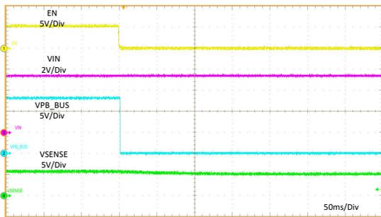
$EN = 5\text{ V to }0\text{ V}$   $PB\_CC1 = R_d$   $I_{PB\_BUS} = 3\text{ A}$
