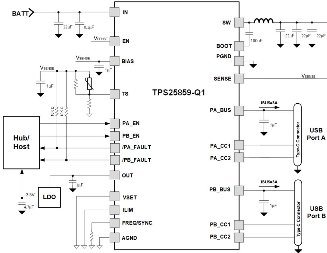
Figure 11-2. TPS25859-Q1 Typical Application Circuit for 400-kHz  $f_{sw}$
