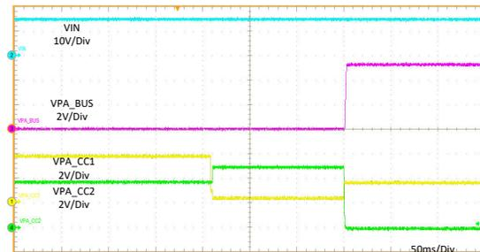
$PA\_CC1 = \text{Open to } R_d$   $PA\_CC2 = \text{Open}$   $I_{PA\_BUS} = 3\text{ A}$
