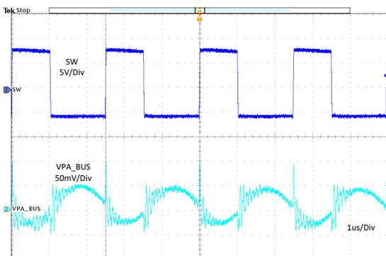
VSET = GND  $I_{PA\_BUS} = 3\text{ A}$   $I_{PB\_BUS} = 3\text{ A}$   $f_{SW} = 400\text{ KHZ}$
