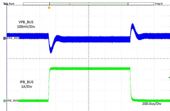
VSET =  $I_{PB\_BUS} = 0\text{ A to }3\text{ A}$   $I_{PA\_BUS} = 3\text{ A}$   $f_{SW} = 400\text{ kHz}$
