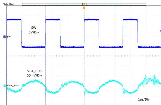
VSET = GND  $I_{PA\_BUS} = 0.1\text{ A}$   $I_{PB\_BUS} = 0\text{ A}$   $f_{SW} = 400\text{ KHZ}$
