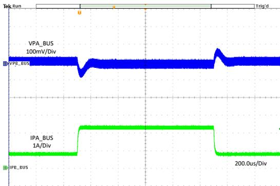
VSET =  $I_{PA\_BUS} = 0.75\text{ A to }2.25\text{ A}$   $I_{PB\_BUS} = 0\text{ A}$   $f_{SW} = 400\text{ KHZ}$
