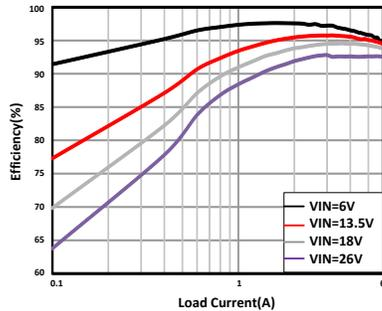
VSET = GND  $f_{SW} = 400\text{ kHz}$   $L = 3.3\text{ }\mu\text{H}$
