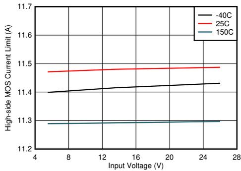
Figure 8-7. High-side Current Limit vs Input Voltage
