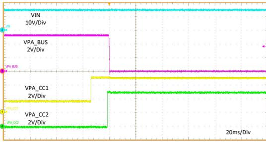
PA\_CC1 =  $R_d$  to Open    PA\_CC2 = Open     $I_{PA\_BUS} = 3\text{ A}$
