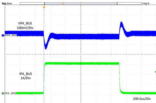
VSET =  $I_{PA\_BUS} = 0\text{ A to }3\text{ A}$   $I_{PB\_BUS} = 3\text{ A}$   $f_{SW} = 400\text{ kHz}$
