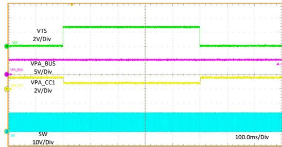
$V_{TS} = 0 \text{ V to } 2.6 \text{ V}$       PA\_CC1 =  $R_d$       PA\_CC2 = OPEN
