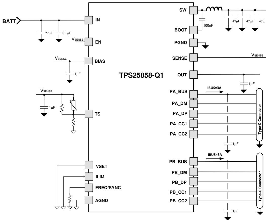
Figure 11-1. TPS25858-Q1 Typical Application Circuit for 400-kHz  $f_{sw}$
