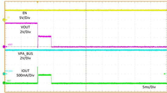
PA\_CC1 =  $R_d$       OUT = 5.1  $\Omega$       PA/B\_BUS NO LOAD
