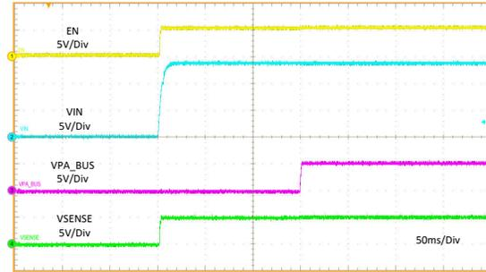
$VIN = 0\text{ V to }13.5\text{ V}$   $PA\_CC1 = R_d$   $I_{PA\_BUS} = 3\text{ A}$
