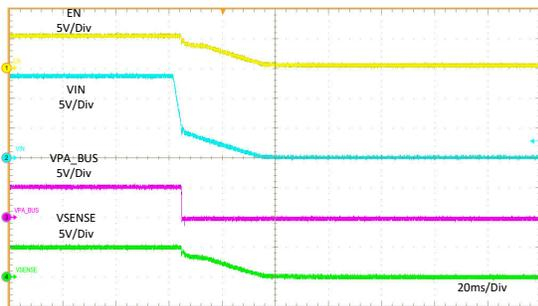
$VIN = 13.5\text{ V to }0\text{ V}$   $PA\_CC1 = R_d$   $I_{PA\_BUS} = 3\text{ A}$
