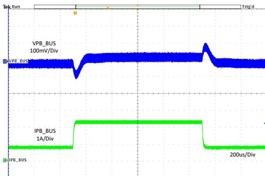
VSET =  $I_{PB\_BUS} = 0.75\text{ A to }2.25\text{ A}$   $I_{PA\_BUS} = 0\text{ A}$   $f_{SW} = 400\text{ KHZ}$
