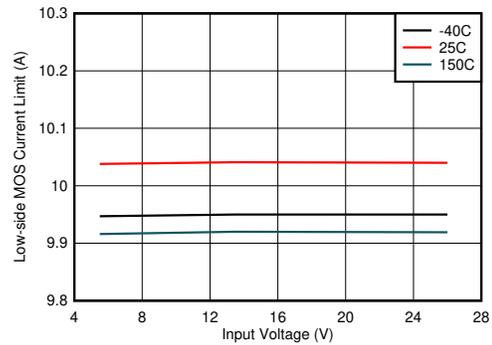
Figure 8-8. Low-side Current Limit vs Input Voltage
