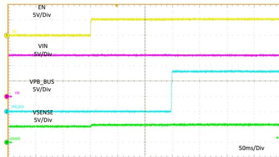
$EN = 0\text{ V to }5\text{ V}$   $PB\_CC1 = R_d$   $I_{PB\_BUS} = 3\text{ A}$
