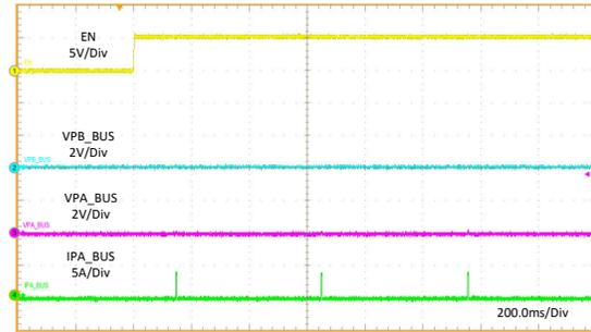
EN to High    PA\_BUS = GND    PB\_BUS = GND
