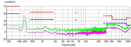
PA\_BUS = 3A,  $f_{SW} = 400\text{ kHz}$   $L = 3.3\text{ }\mu\text{H}$
