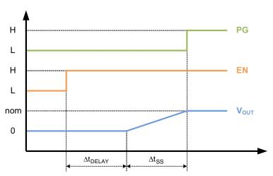
Figure 8. Soft-Start Timing ( $\Delta t_{SS}$ )
