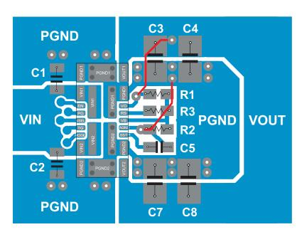
Figure 41. TPSM82480 Board Layout
