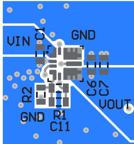
Figure 8-60. PCB Layout Recommendation (RDS Package)
