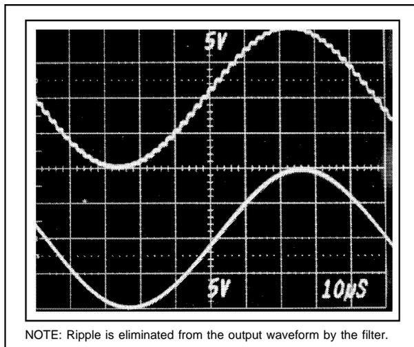
NOTE: Ripple is eliminated from the output waveform by the filter.
