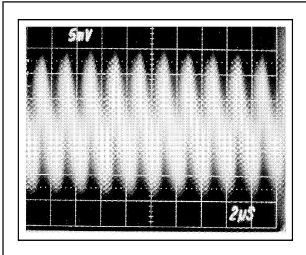
FIGURE 3. Standard ISO122 (approximately 20mVp-p output ripple).
