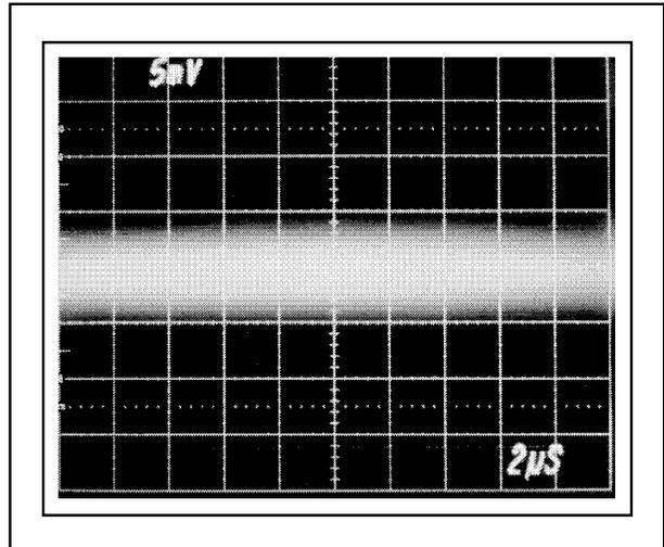
FIGURE 4. Filtered ISO122 (no visible output ripple).
