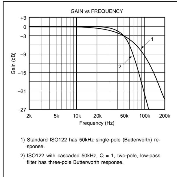
FIGURE 2. Gain vs Frequency Plot.
