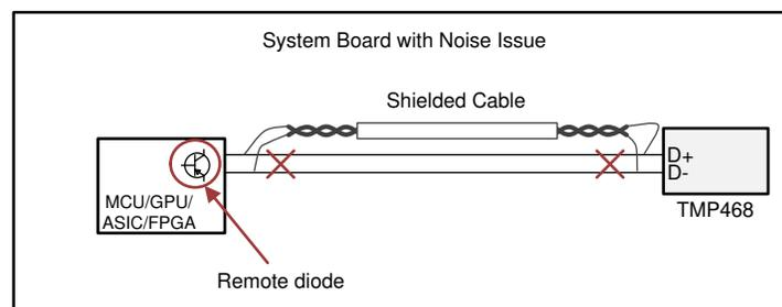
**Figure 22. Isolating Noise Coupling Into Remote Transistor Traces**
