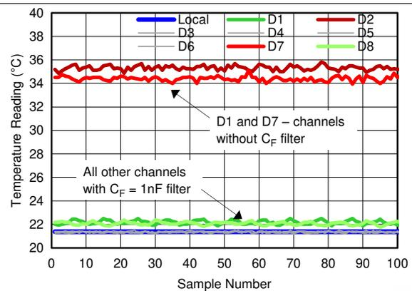
**Figure 19. TMP468EVM Noise Level Measurement With Noise Injection**
