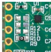
**Figure 7. EVM Address Pin Hole Connections**
