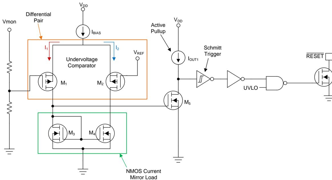
Figure 6. Undervoltage Only Supervisor Architecture
