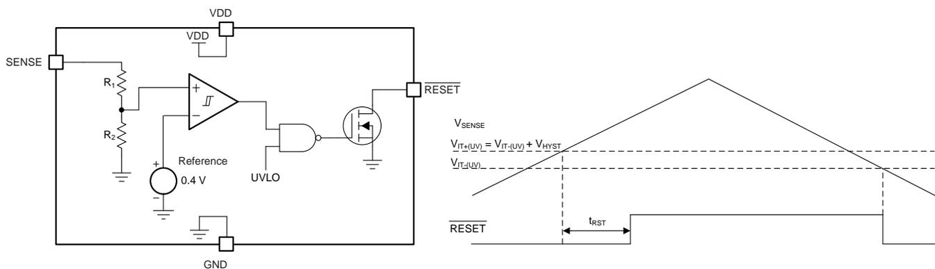
**Figure 1. Undervoltage Supervisor Block Diagram and Timing Diagram**
