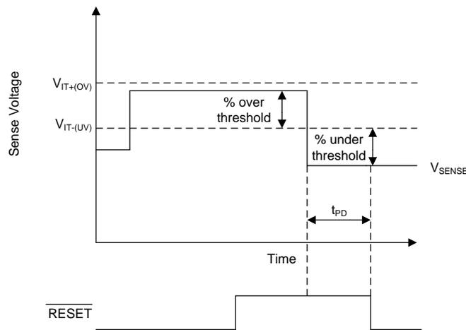
Figure 9. Measuring the Overdrive Voltage Curve
