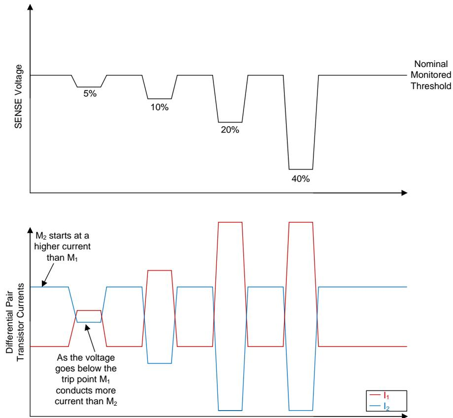
**Figure 11. Differential Pair Current During Normal Use**
