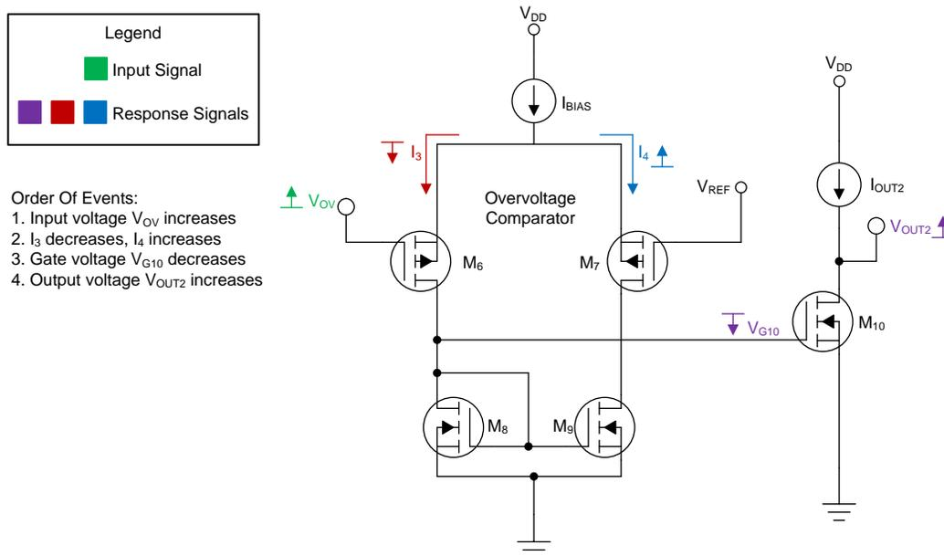
Figure 8. Overvoltage Comparator Signal Tracing
