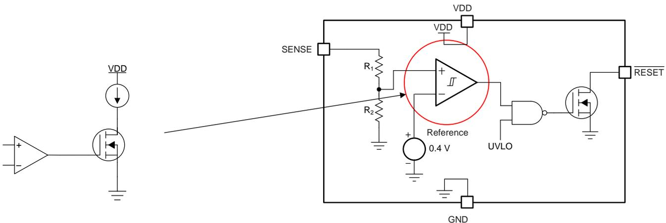
Figure 3. Comparator with Active Pullup Current Source
