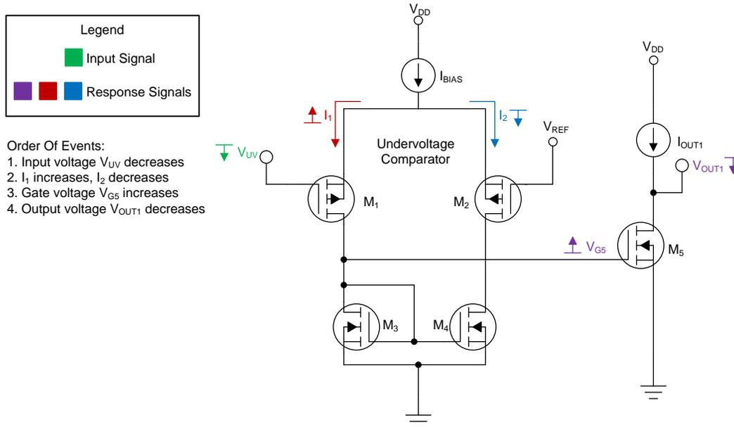
Figure 7. Undervoltage Comparator Signal Trace
