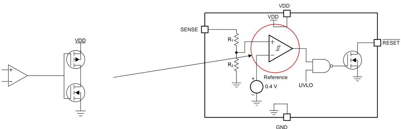
Figure 4. Comparator with Push-Pull Output
