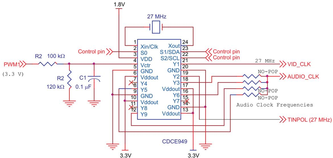
Figure 4. Single-Chip Solution to Generate Synchronized Video and All Audio Frequencies
