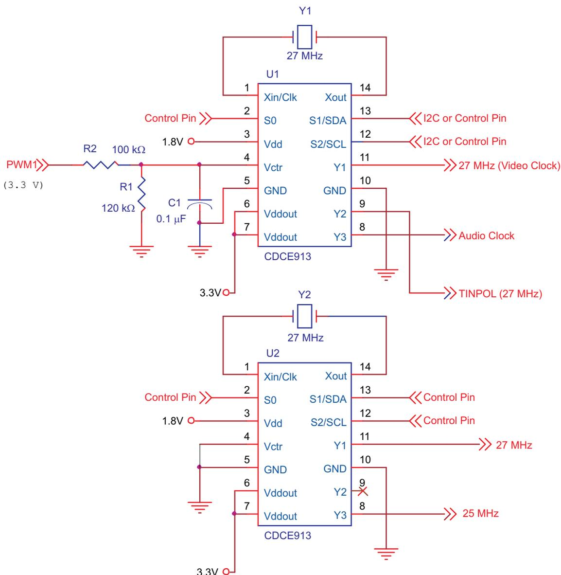
**Figure 3. Two-Chip Solution to Generate All Frequencies for this System**
