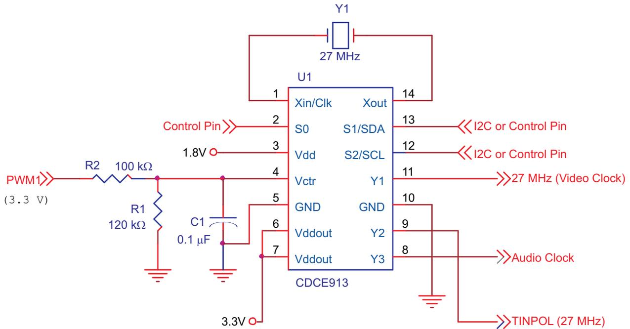
**Figure 2. Single-Chip Solution to Generate Synchronized Audio and Video Clock Frequencies**
