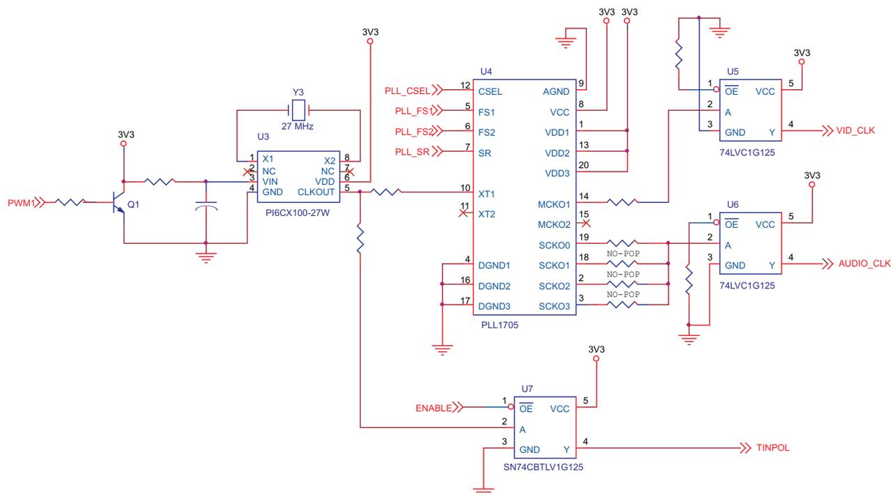
**Figure 1. Generating Synchronized Video and Audio Clocks (The Current Clocking Proposal With Several ICs)**
