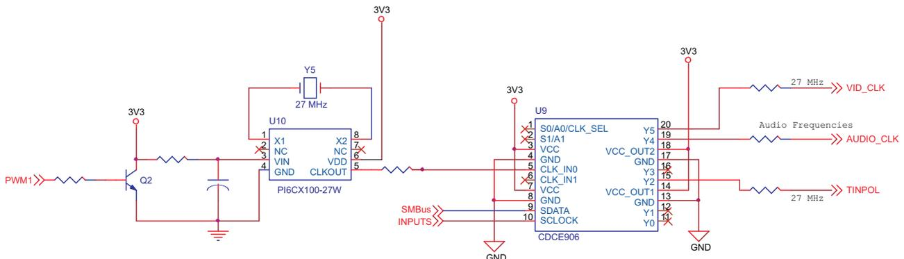
Figure 5. Two-Chip Solution Using SMBus Interface Programming
