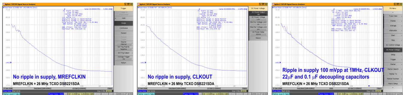
Figure 9. CDC3S04 Additive Jitter When Sweeping the Ripple in the Power Supply in Frequency and Amplitude
