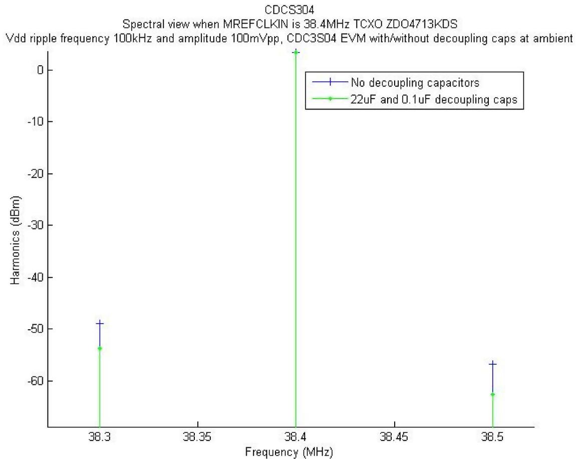
**Figure 8. CDC3S04 Frequency Spectrum With Supply Ripple of 50-mVpp Amplitude and 100-kHz Frequency**
