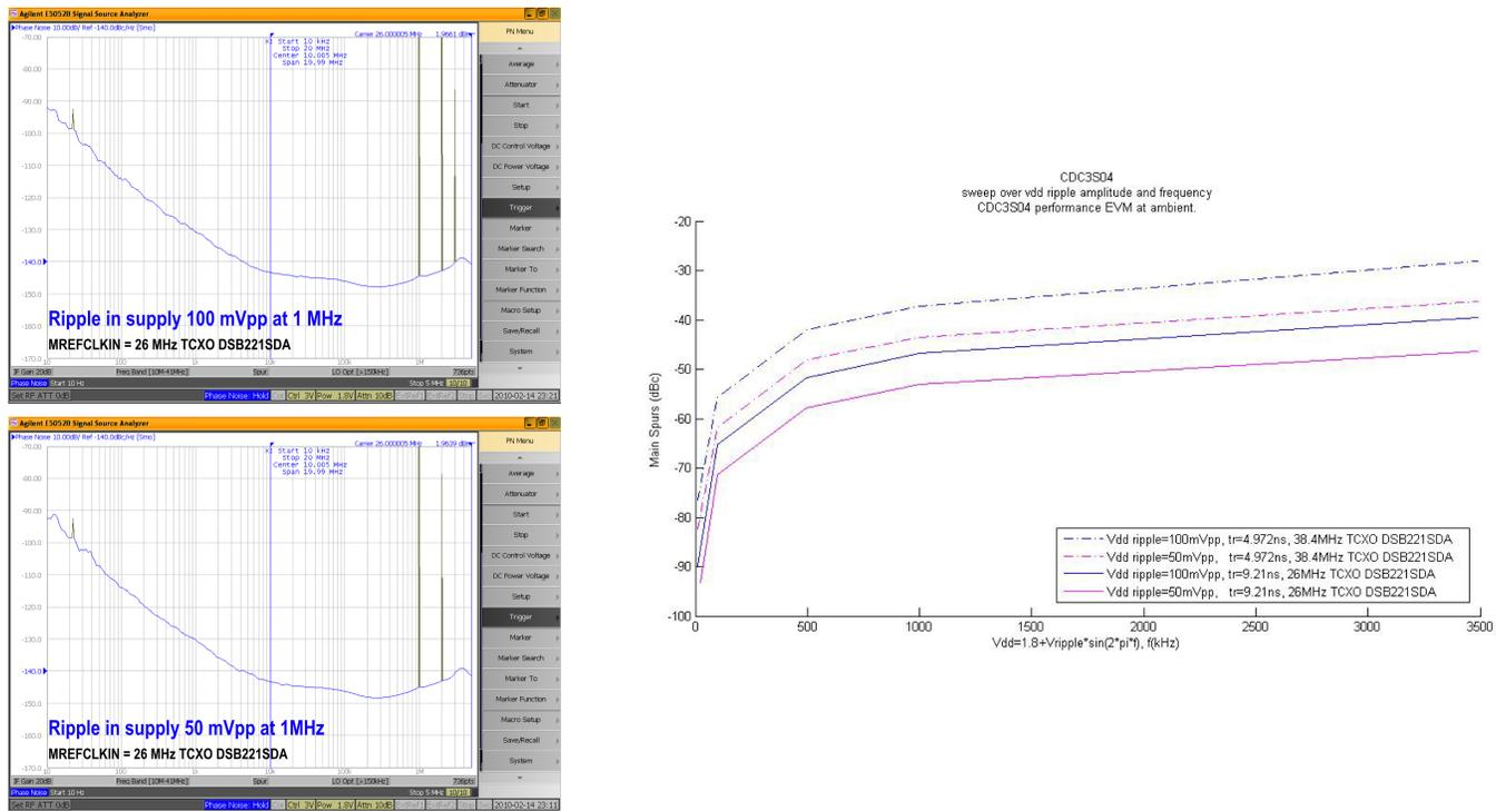
Figure 4. CDC3S04 Main Spurs Variance With Vdd Ripple Amplitude and Frequency, CLKIN = 26-MHz TCXO and 38.4-MHz TCXO DSB221SDA
