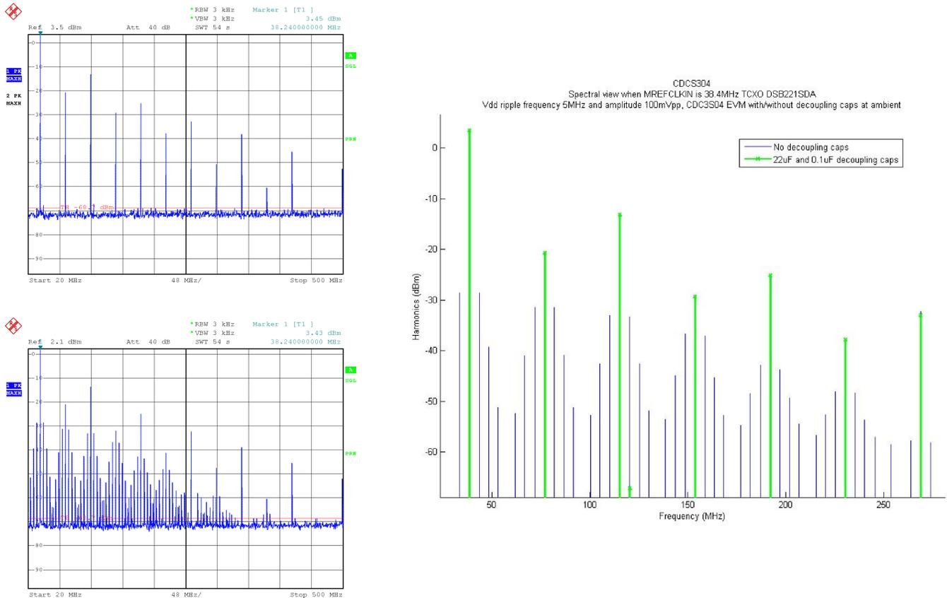
Figure 7. CDC3S04 Frequency Spectrum With Supply Ripple of 100-mVpp Amplitude and 5-MHz Frequency
