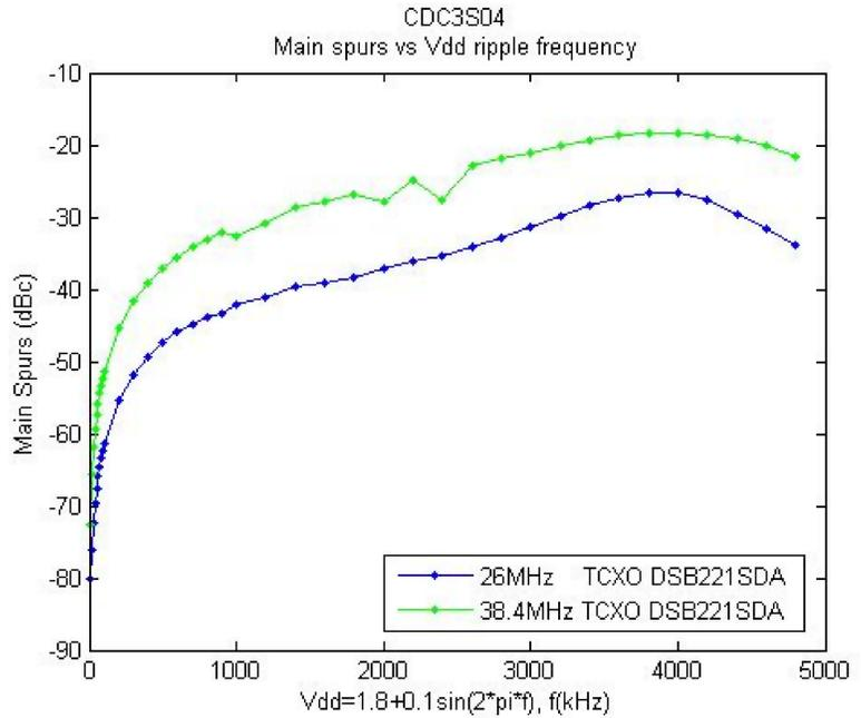
Figure 2. CDC3S04 Main Spurs, Vdd = 1.8-Vdc Signal + Variable-Frequency Sinusoidal
