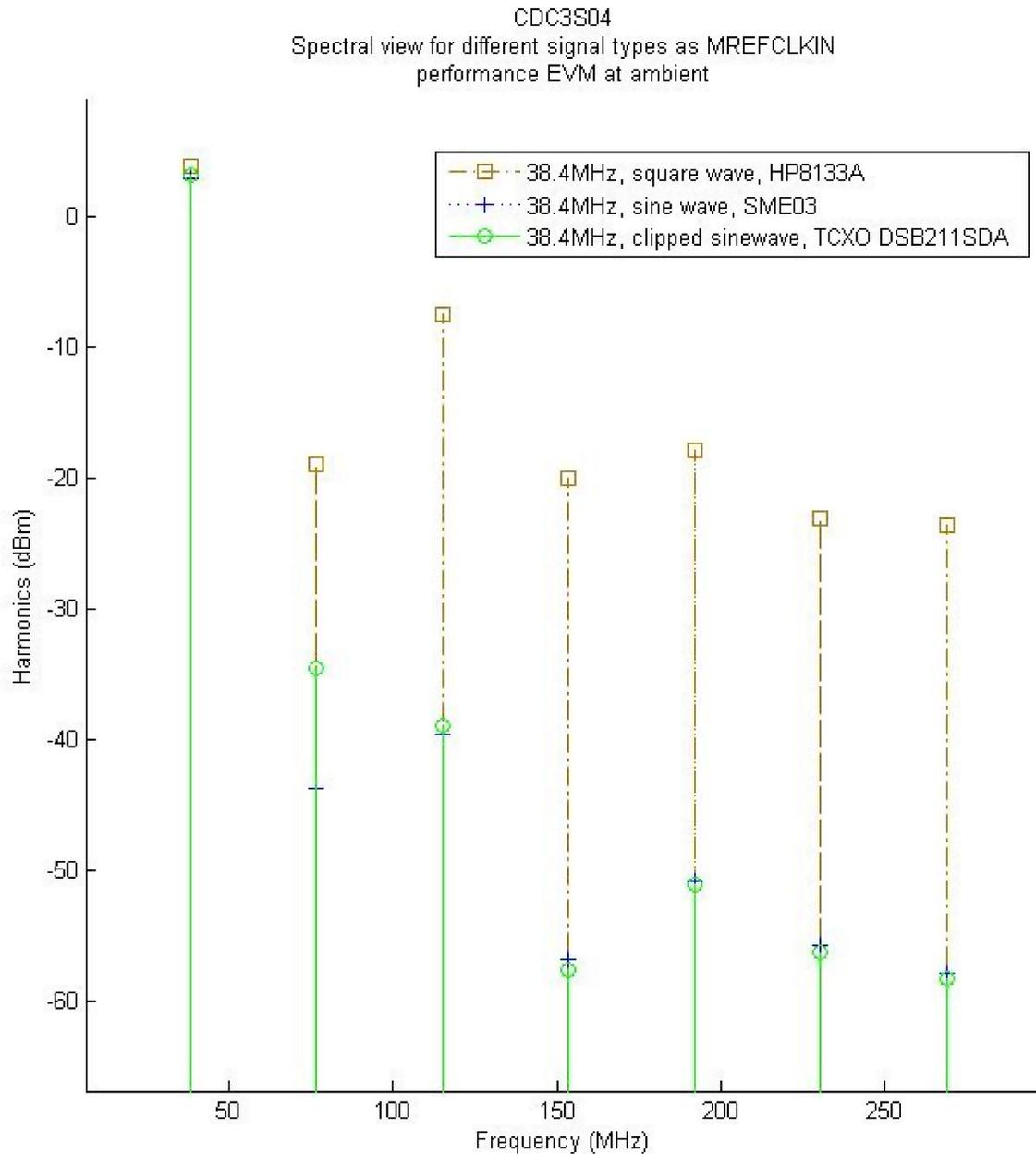
**Figure 1. CDC3S04 Spectral View Comparison: Square Wave, Sine Wave, and Clipped-Sine Wave**
