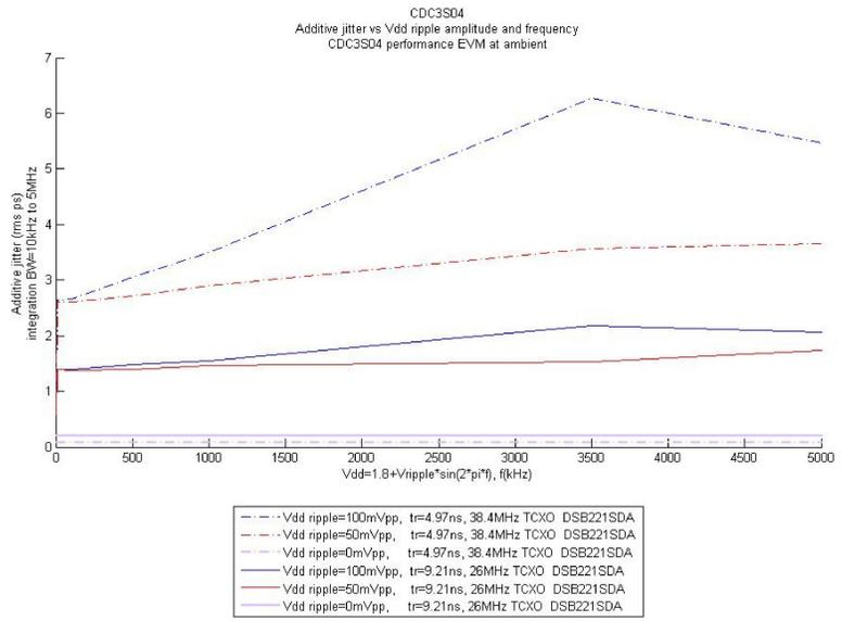
Figure 5. CDC3S04 Additive Jitter for Integration Bandwidth of 10 kHz to 5 MHz, Vdd Ripple Amplitude and Frequency Varied for Different Clock Inputs: 26-MHz TCXO and 38.4-MHz TCXO DSB221SDA
