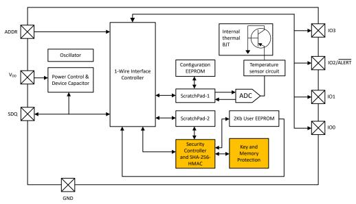
Figure 1-1. Functional Block Diagram
