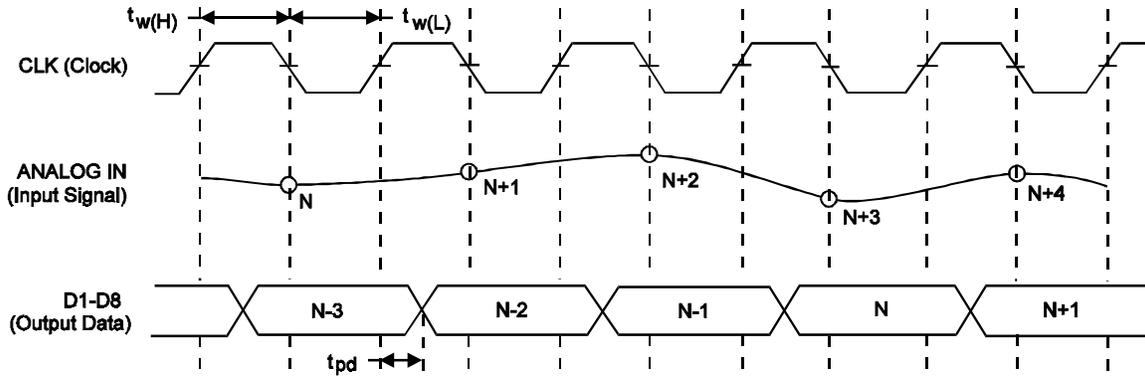
The digital data is valid after a delay time  $t_{pd} = 30$  ns for the TLC5510. Table 1 summarizes important TLC5510 parameters.
