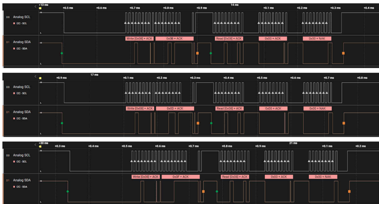
Figure 4-3. Captured I2C Waveform for PF Status Reading
