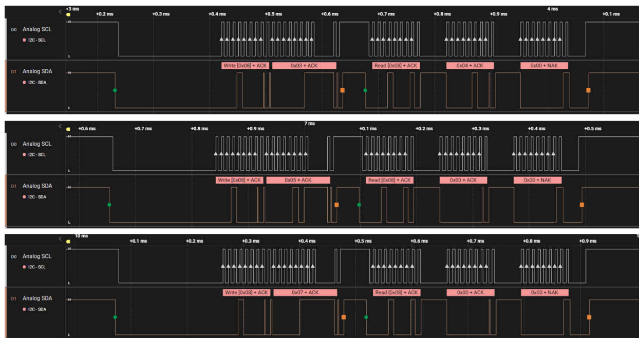
Figure 4-2. Captured I2C Waveform for Safety Status Reading
