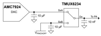
Figure 3-2. Recommended Output Switching Capacitors
