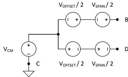
**Figure 6. Resistive Bridge Output Voltages**
