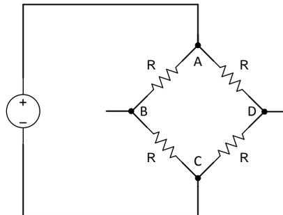
Figure 2. Resistive Bridge Sensor Without Pressure Applied
