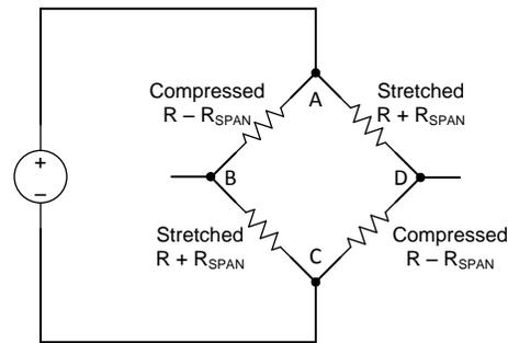
**Figure 3. Resistive Bridge Sensor With Pressure Applied**
