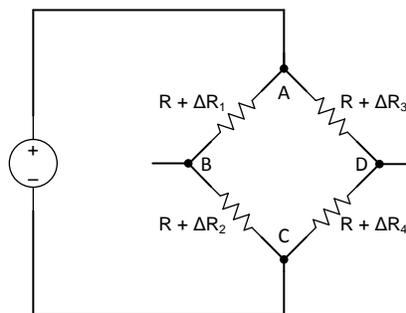
Figure 5. Real Resistive Bridge Sensor Without Pressure Applied
