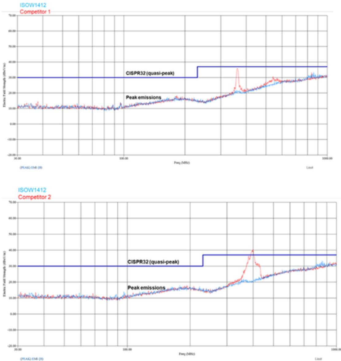
**Figure 4. Emissions comparison of ISOW1412 and 2 competing devices. ISOW1412 meets CISPR 32 Class B emissions mask on a 2 layer board**
