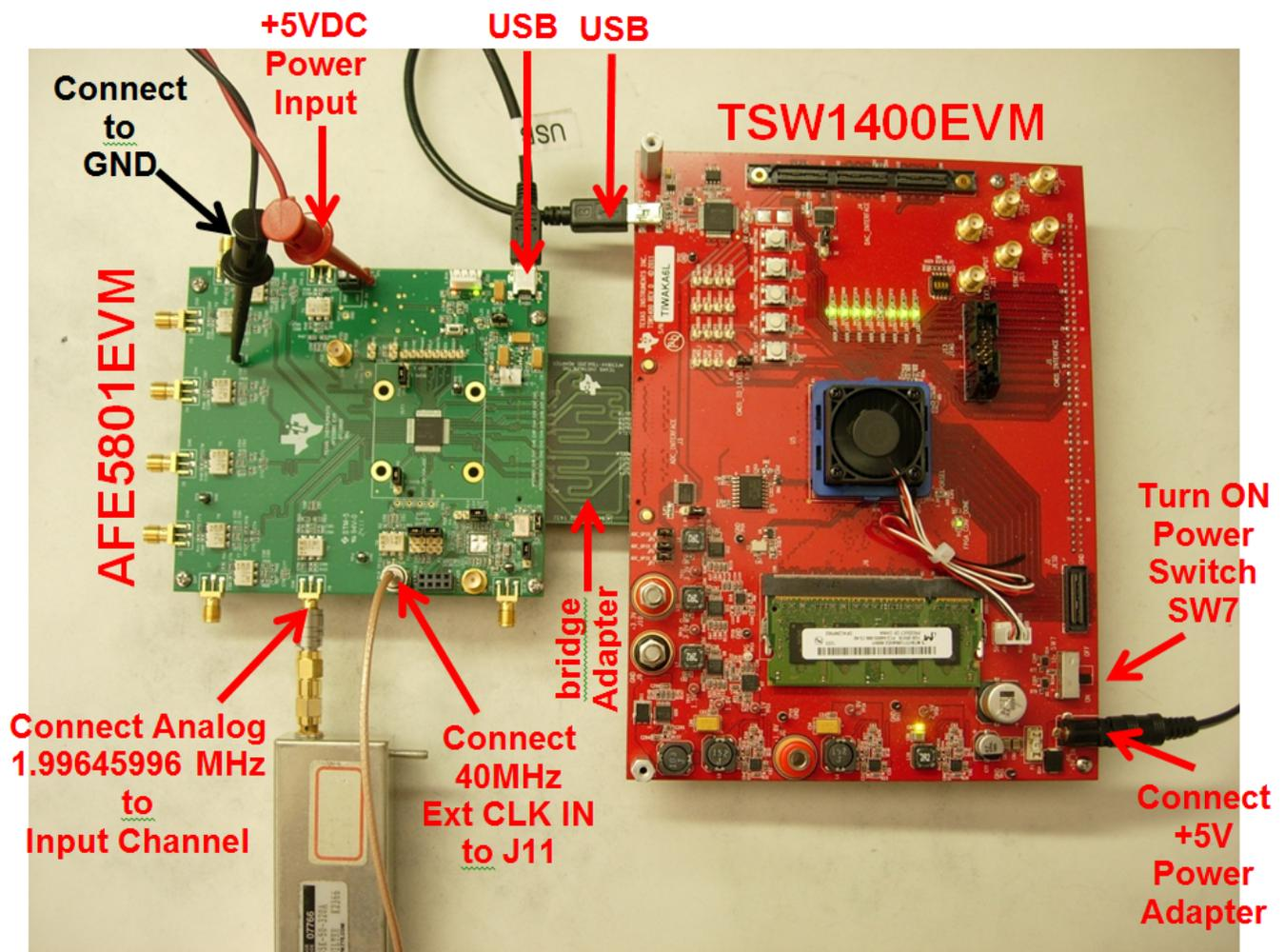
Figure 29. Connection Between TSW1400EVM and AFE5801
