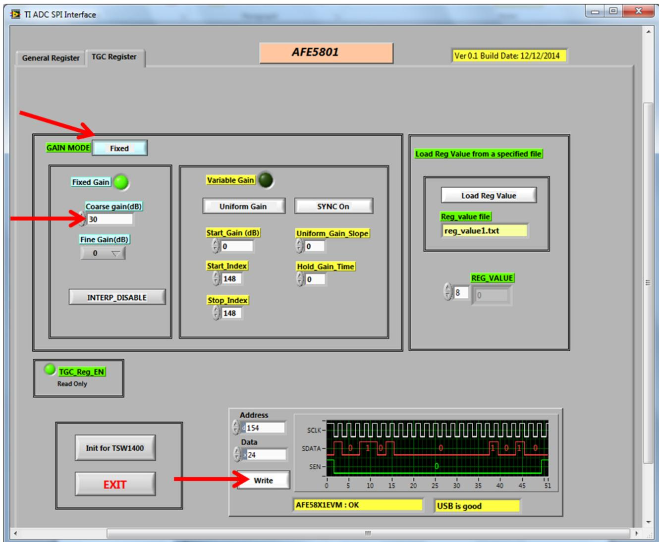
Figure 34. AFE5801EVM GUI - Setting Fixed Gain
