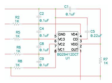
Figure 16. bq29412 Cell Inputs and Time-Delay Capacitor
