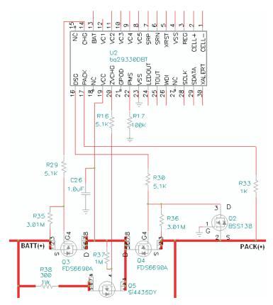
Figure 14. PACK, VCC, PMS Inputs, and FET Control
