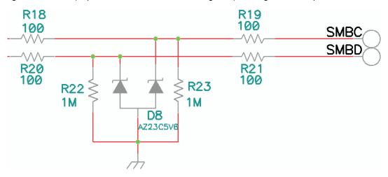
Figure 9. ESD Protection for SMB Communication
