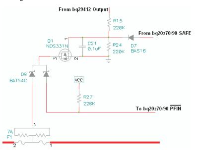
Figure 10. SAFE Circuit
