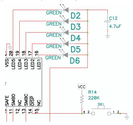
Figure 5. LEDs and Display Switch
