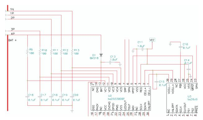
Figure 13. Cell and BAT Inputs
