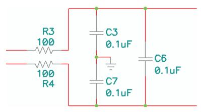
Figure 6. Differential Filter
