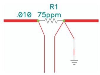
Figure 4. Sense Resistor
