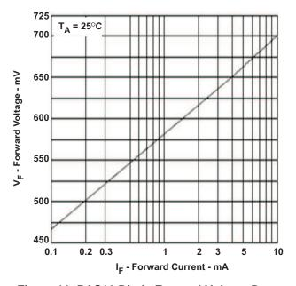
Figure 11. BAS16 Diode Forward Voltage Drop
