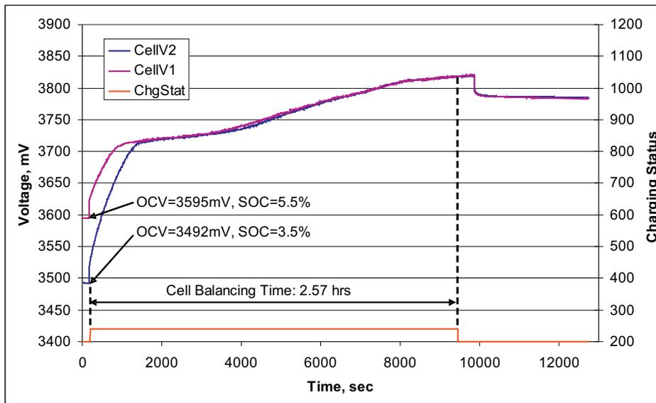
Figure 3. Fast Cell Balancing of Two Series Cells
