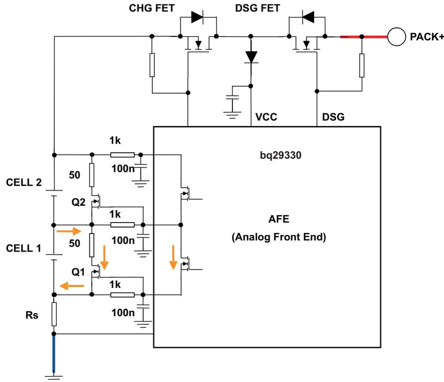
Figure 2. External Cell-Balancing Circuit With Cell 1 Bypassing Active
