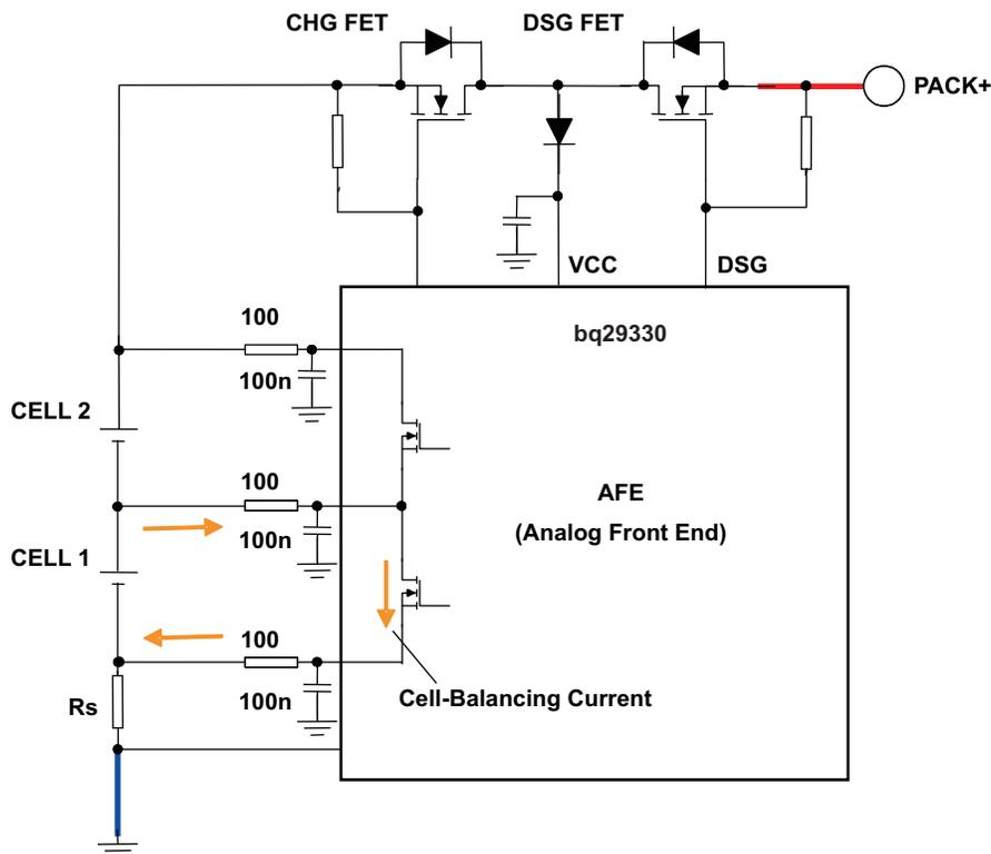
**Figure 1. Internal Cell-Balancing Circuit of bq29330 AFE**
