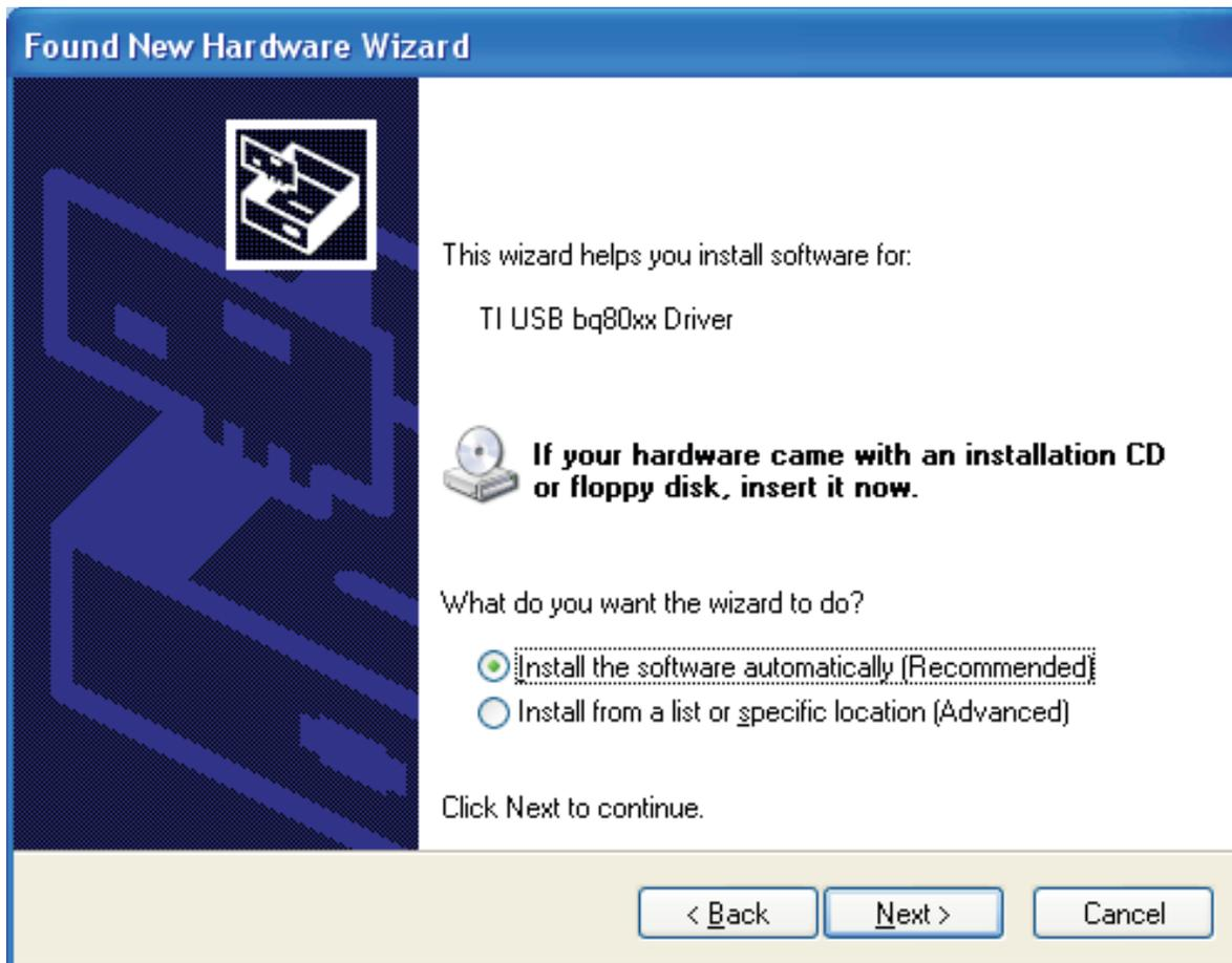
7. Select **Install the software automatically (Recommended)** and click Next on the next Found New Hardware screen for the second of the 2 drivers (TI USB bq80XX Driver) required for this instance of the EV2300.
