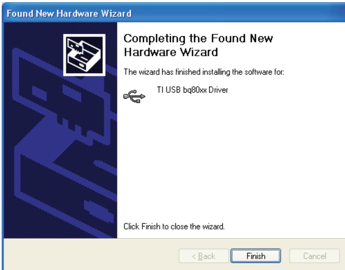
10. The TI bq80XX Driver is now installed for this instance of the EV2300. Click **Finish** to exit the driver install wizard.
