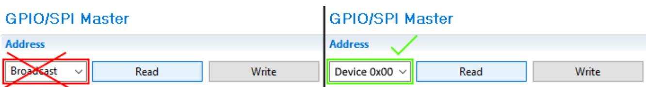
**Figure 21. SPI Master Command Frame Change**
