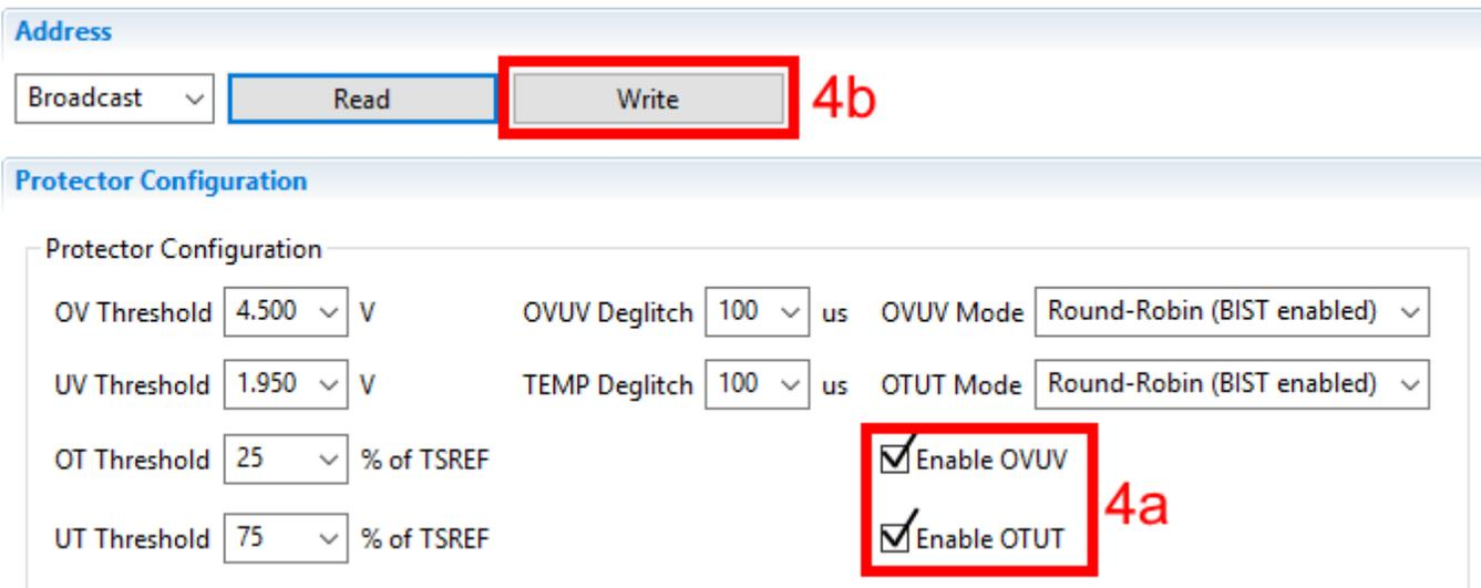
Figure 27. Enable OVUV and OTUT
