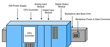
Figure 1. Example of a Typical PLC System
