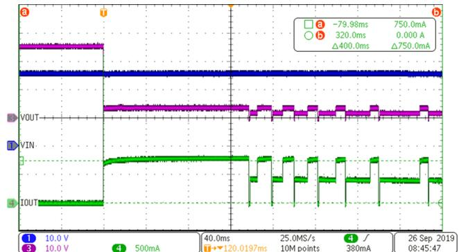
Figure 3. Waveform of the TPS27S100 During an Overload Condition (5- $\Omega$  / 4.2-A Load)
