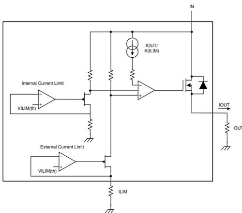
Figure 2. TPS27S100 Adjustable Current Limit Functional Block Diagram
