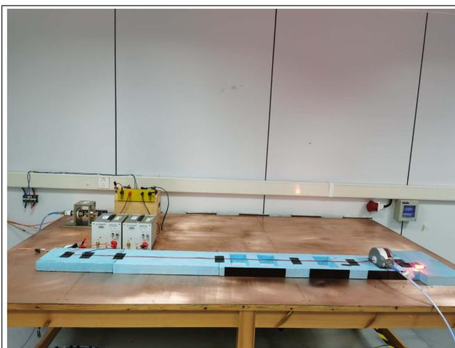
Figure 4. General Setup of BCI Test
