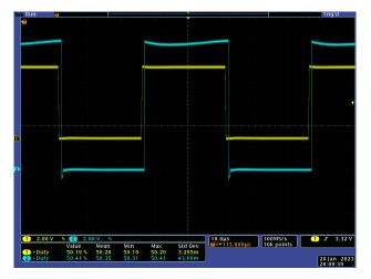
Figure 5. DRV8311H Measured Duty Cycle at 50.2%
