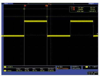
Figure 2. DRV8311P Measured Duty Cycle at 50.0%
