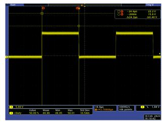
Figure 3. DRV8311P Measured Duty Cycle at 50.2%
