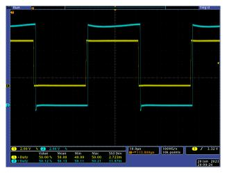
Figure 4. DRV8311H Measured Duty Cycle at 50.0%
