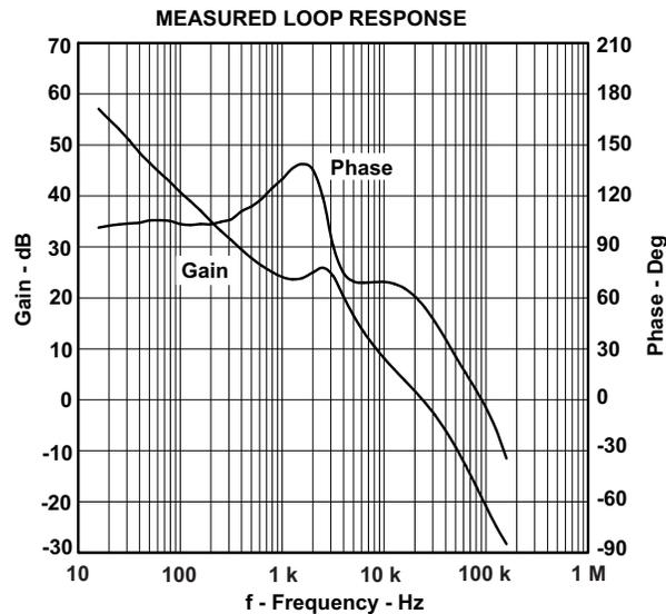
Figure 5. Measured Loop Response, TPS5420, VIN = 25 V
