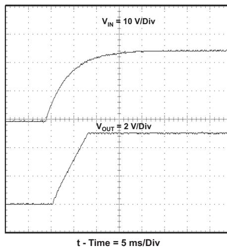
Figure 8. Power Up,  $V_{OUT}$  Relative to  $V_{IN}$
