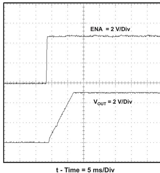
**Figure 9. Start-Up Waveform, V<sub>OUT</sub> Relative to ENA**
