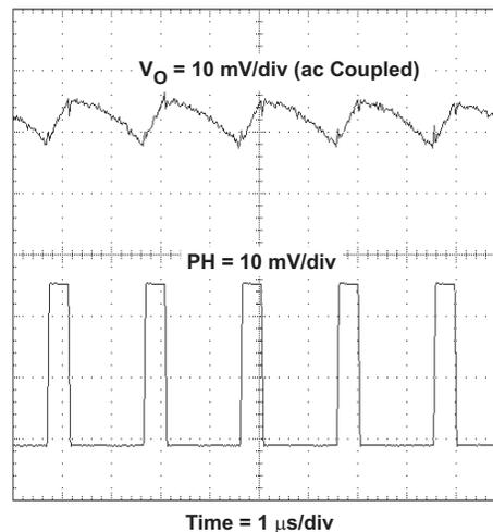
Figure 6. Measured Output Voltage Ripple, TPS5420
