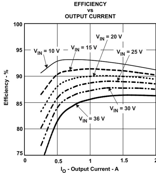
Figure 1. Measured Efficiency, TPS5420
