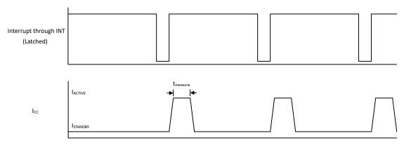
Figure 2-4. Timing Diagram for Conversion on Demand
