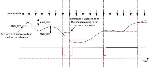
Figure 2-7. TMAG3001 Wake on Change with Angle Measurements
