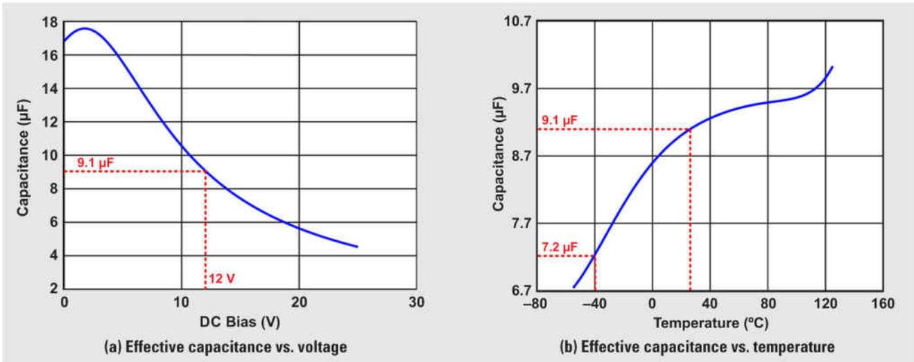
Figure 4. MLCC Plots for a 22-µF, 25-V, 1210, X7R Capacitor
