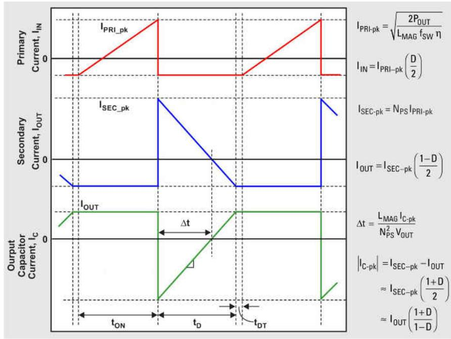
**Figure 3.** Idealized Current Waveforms of a Flyback Converter in BCM
