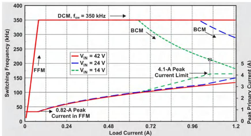
**Figure 2.** Switching Frequency and Primary Peak Current vs. Load Current for the LM25184
