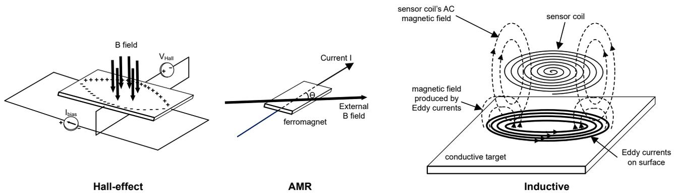
**Figure 1.** Hall-effect, AMR and inductor sensor functionality.
