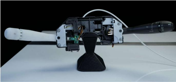
**Figure 2.** Steering column retrofitted with TI 3D sensor evaluation modules.
