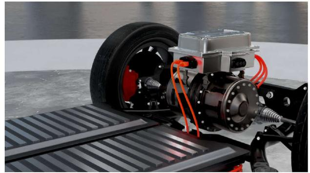
**Figure 3.** Electric motor and traction inverter.
