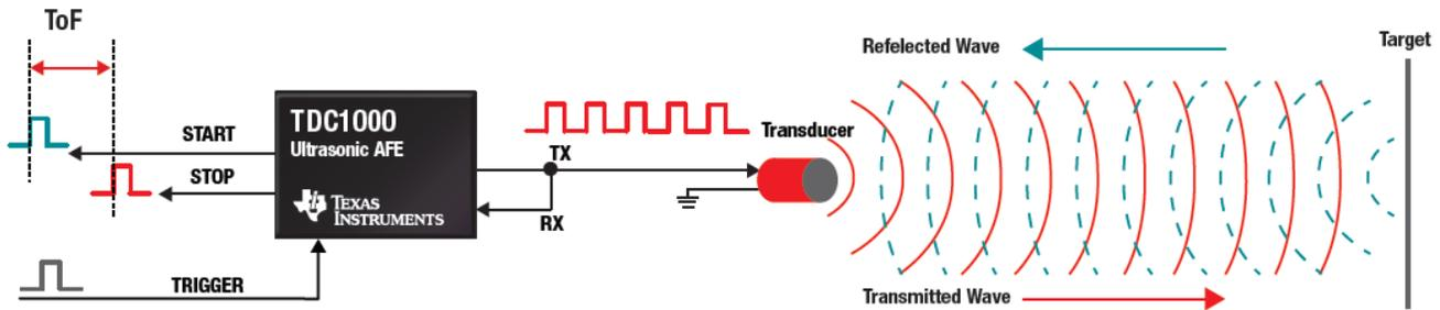
**Figure 1. How Ultrasonic Works for Single Transducer Measurement**
