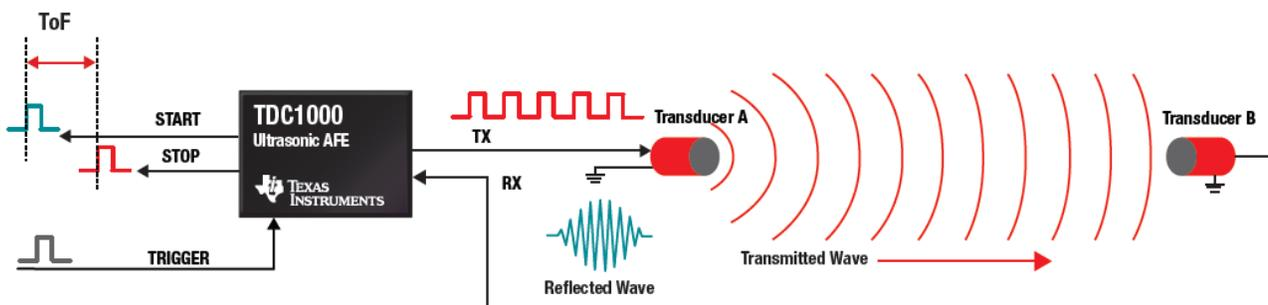
**Figure 2. How Ultrasonic Works for Dual Transducer Measurement**
