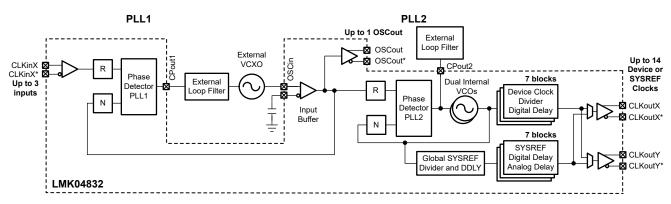
Figure 1-1. LMK04832-SEP Configured in Dual-Loop Mode
