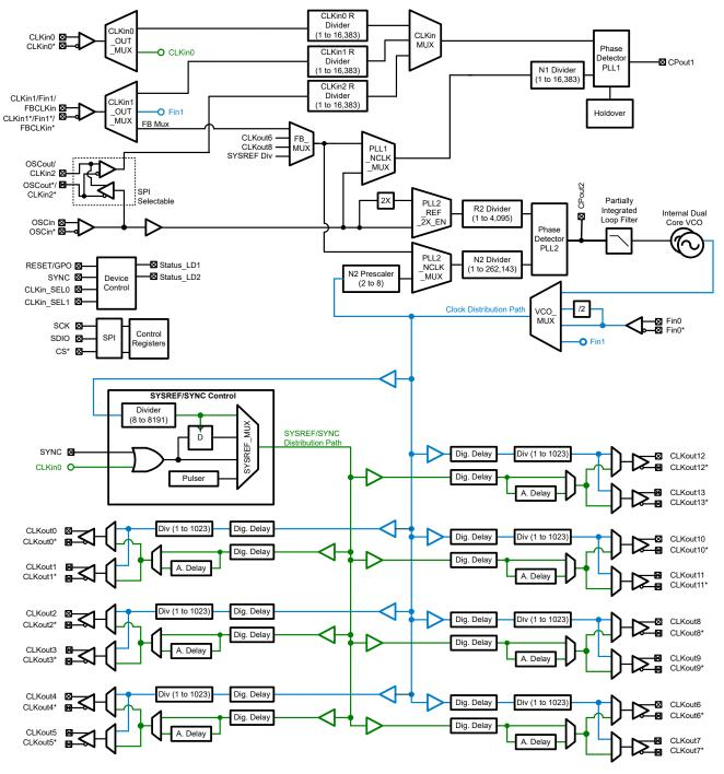
Figure 1-2. LMK04832-SEP Detailed Block Diagram
