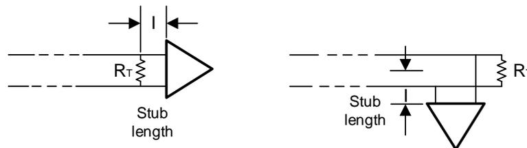
**Figure 5. Termination Layout Standard and Fly-by**
