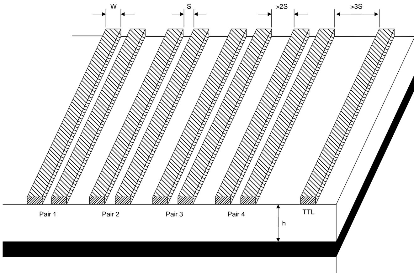
**Figure 4. Differential Trace Spacing**
