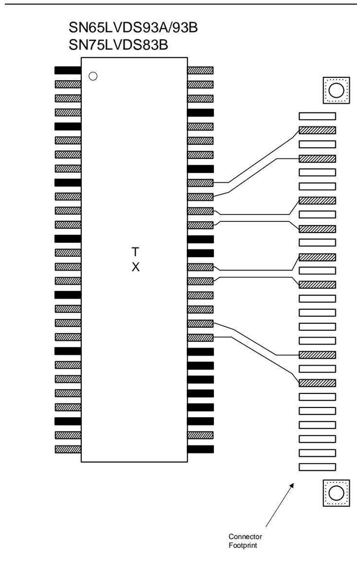
Figure 3. LVDS PCB Layout
