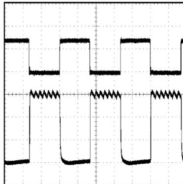
$I_{LED} = 6A$  nominal,  $V_{IN} = 3.3V$ ,  $V_{EE} = -12V$  Top trace: DIM input, 2V/div, DC Bottom trace:  $I_{LED}$ , 2A/div, DC T = 10 $\mu$ s/div
