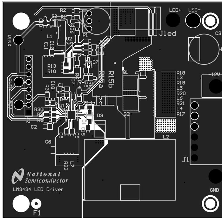
Figure 6. Top Layer and Top Overlay
