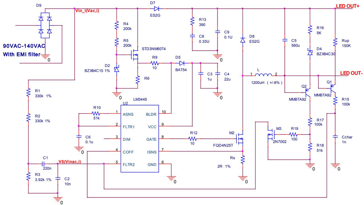
Figure 1. Traditional Proposed Nonisolated Solution With High PF
