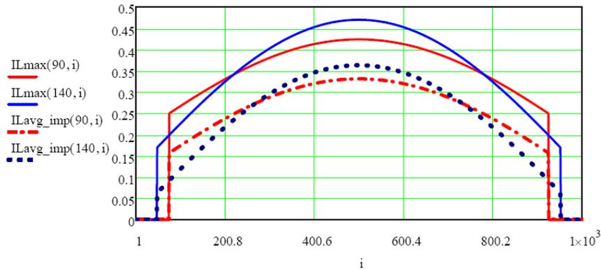
Figure 14. Inductor Current Less Than 90 Vac and 140 Vac
