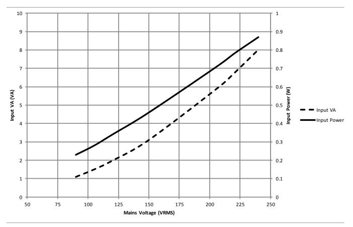
Figure 8. Actual Power and Apparent Power Vs Line Voltage
