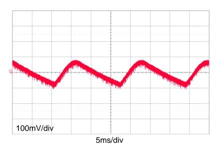
Figure 3. Voltage Ripple at  $V_{DC}$
