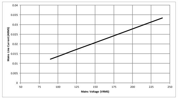
Figure 7. Line Current Vs Line Voltage
