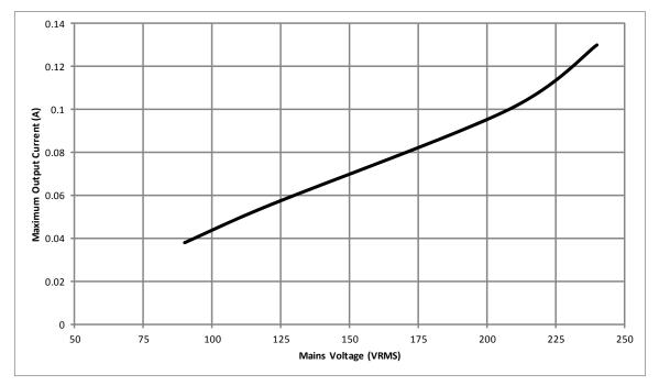
Figure 6. Max Output Current vs Line Voltage
