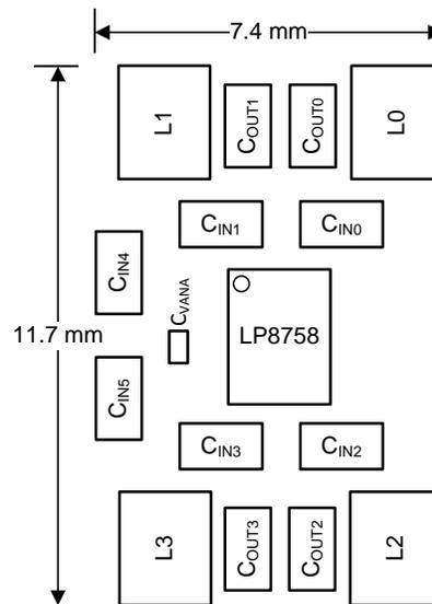
Figure 6. Component Placement near the LP8758 Device
