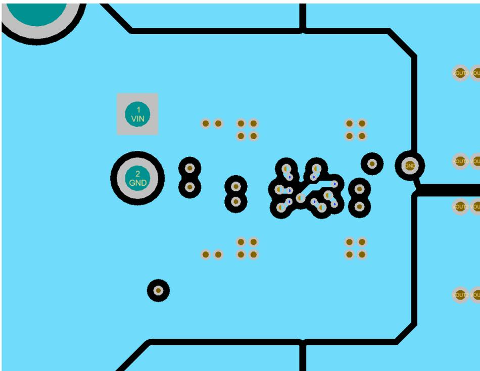
Plane kept intact around the LP8758 device.
