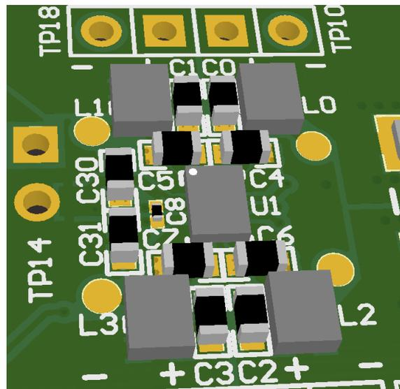
Figure 11. 3D view Showing the LP8758 Device and Nearest Components
