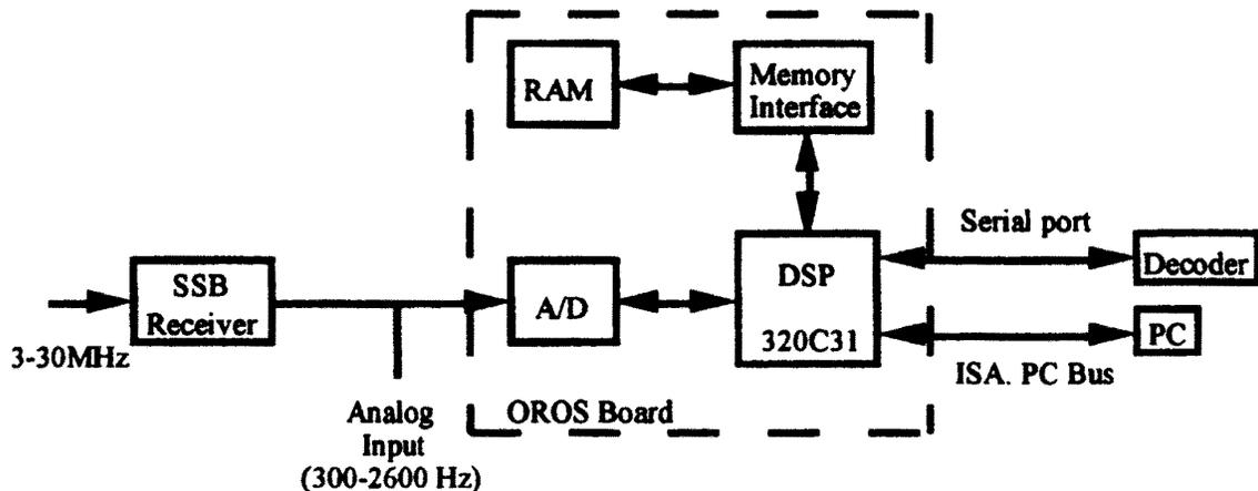
To test the MODEM transmitter, random data is sent from the DSP through the ISA PC bus. Handled data files are sent back to the PC. The DSP output data is converted from digital to analog and the analog output is then used to test the transmission. The data is subsequently up-converted and sent through the ionospheric channel.
