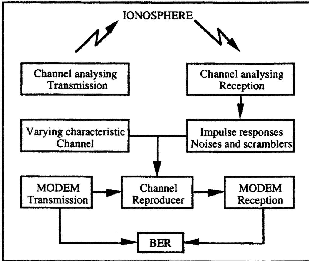
The first method uses varying characteristic channels, the second one uses impulse responses measured on experimental channels. In both methods, a channel reproducer is used to simulate the whole transmission.
